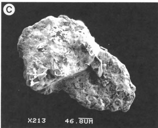
Figure 21. Scanning electron microscope photomicrographs of gold grains recovered from pan concentrates of tills at the Forest Hill Gold District. Magnification and bar scales are shown on each photograph.
