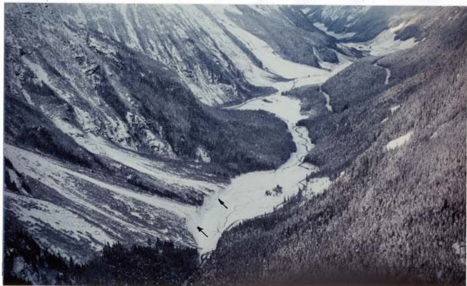
PL VB. Photo taken from the same vantage point as PL VA (October 30, 1984). Note the erosion scarps in the valley side fans, the stripped valley bottom vegetation and widened foreground channel. Photo: K. Ricker
