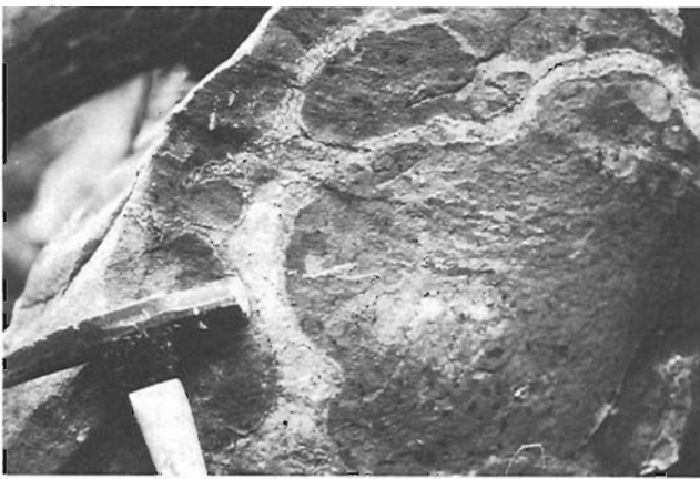
Figure 4. Pillow-like structures exhibited by basalt included in pink, medium grained granite. Note that there is a thin intermediate composition reaction rim on the inclusions; Mount Auclair trail. (GSC 204123-G)
