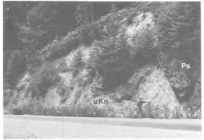
Figure 67.5. Upper strand of the Beaufort Range Fault Zone on Highway 4 near Port Alberni. The man (K. Dom) has his hand on the breccia zone immediately adjacent to the fault which dips easterly at 45^\circ . Ps = Paleozoic Sicker Group. uKn = Upper Cretaceous Nanaimo Group.
