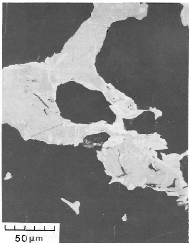
Figure 2. Irregular polycrystalline \beta -domeykite with selvage of idiomorphic loellingite in siliceous gangue.
