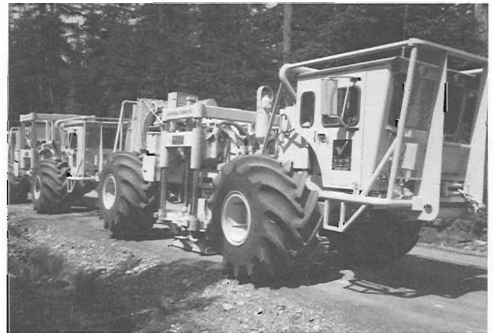
Figure 67.14. Vibrator trucks at the beginning of line 1 near Bamfield.
