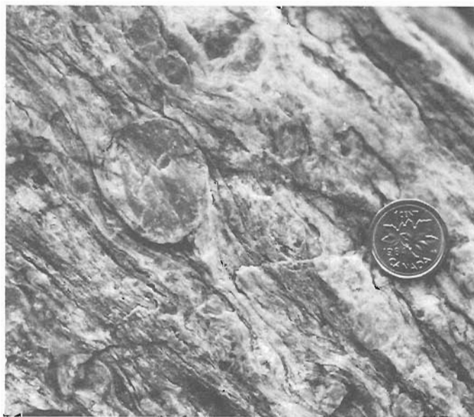
Figure 57.12. Rolled feldspar augen with 'tails' in mylonite derived from pegmatite and syenite (unit E). Plane of photograph is X-Z section. Reverse displacement is indicated.
