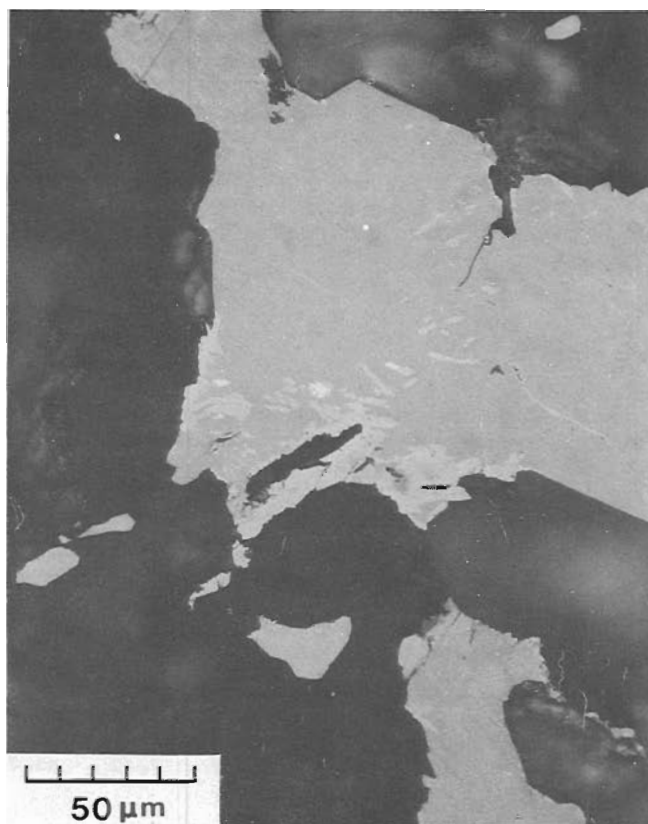
Figure 3. \beta -domeykite with inclusions of native silver and idiomorphic to lamellar grains of loellingite.
