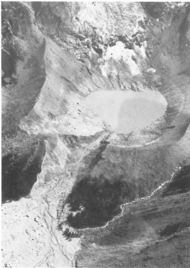
Figure 35: Nostetuko Lake and the breached late Neoglacial end moraine of Cumberland Glacier in the southern Coast Mountains of British Columbia. The lake drained catastrophically in July 1983 when a wave overtopped the moraine. Escaping waters rapidly cut down through the loose morainal debris, producing an alluvión . Photo courtesy of British Columbia Hydro and Power Authority.
