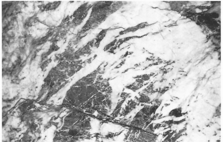
Figure 12. 11 Volcanic-Associated Vein and Shear Zone Gold. Kerr-Addison mine, Virginiatown, Ontario. Typical, irregular gold-bearing quartz veins of the green carbonate zone. Width of field of view is about 1.5 m. Photo: R.V. Kirkham (GSC 203633-S).
