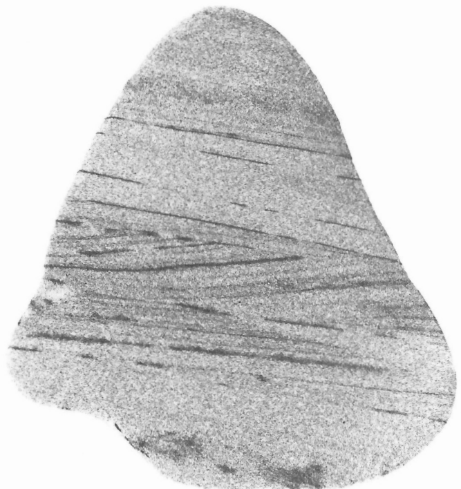
Figure 8. 6.2 Sandstone Lead. Yava deposit, Nova Scotia. Galena and carbonaceous material (mainly wood trash) oriented parallel to bedding in crossbedded terrigenous sandstone. Wood trash is detrital; galena occurs as cement between quartz grains. Sample is approximately 20 cm high. Sample: R.V. Kirkham (GSC 203641-S).
