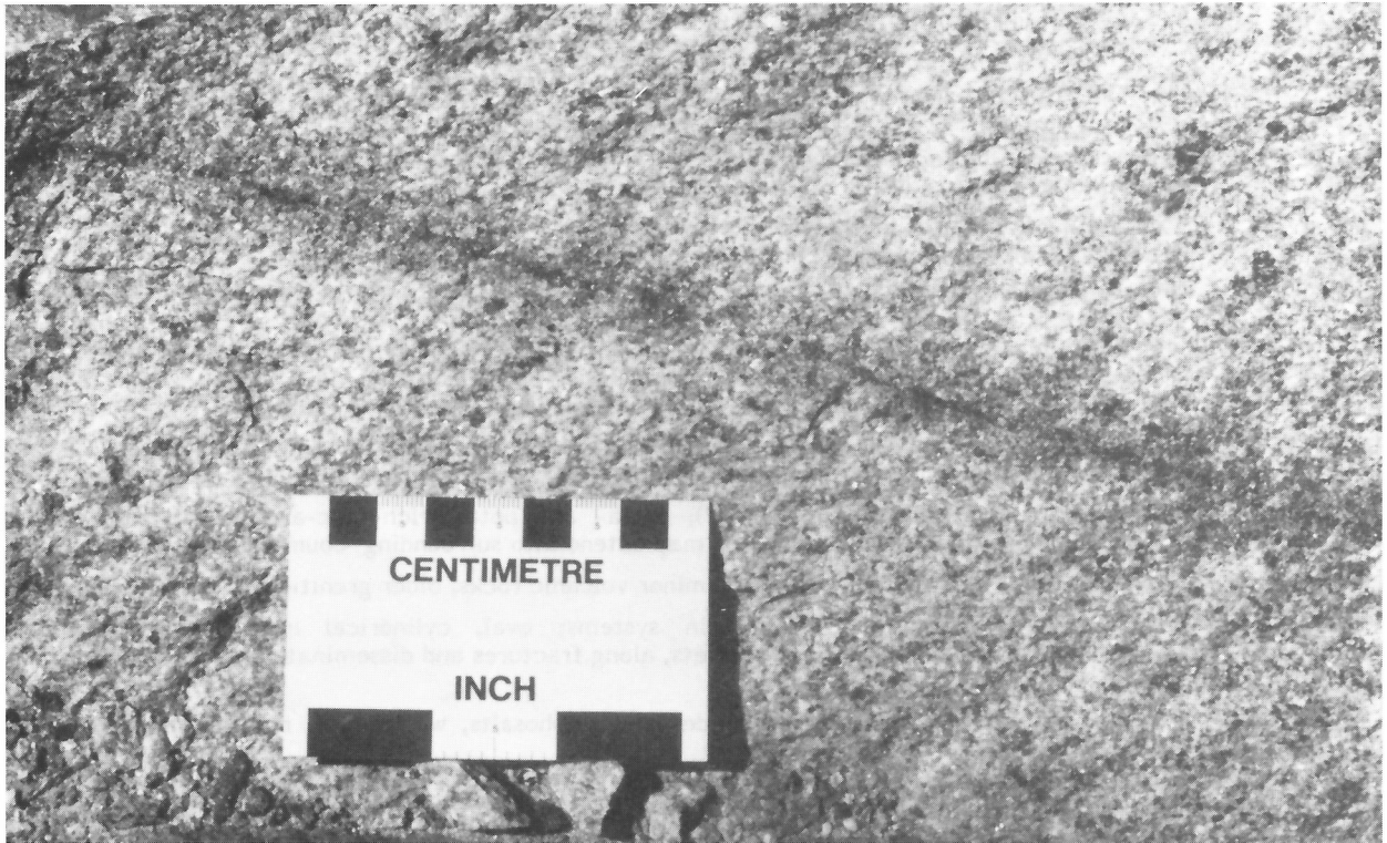
Figure 22. 18 Vein-Stockwork Tin. East Kemptville, Nova Scotia. Greisenized zone of quartz, topaz and muscovite forms an alteration envelope approximately 2 cm wide around a quartz veinlet cutting sericitized granite, East Kemptville tin deposit. Such zones contain cassiterite, as well as pyrite, sphalerite, chalcopyrite, pyrrhotite, minor wolframite and other sulphide minerals. Photo: W.D. Sinclair (GSC 203886-Q).
