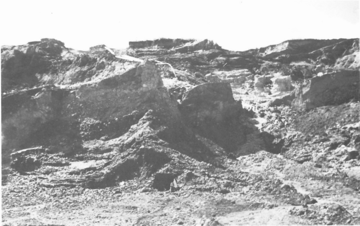
Figure 6. 5.2 Placer Gold. Klondike area, Yukon. Basal part of high level White Channel bench gravels. Early placer miners (c.1902) followed lower bedrock surface with timbered drift (about 1.2 m wide). Bench mined hydraulically and with bulldozer in 1960. Photo: C.R. McLeod (GSC 202282-V).
