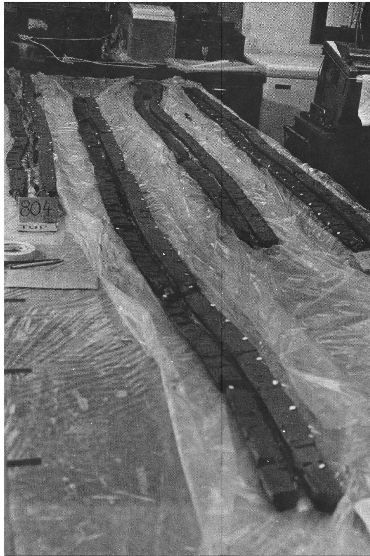
Extruded core lies on laboratory table onboard ship, and has been split lengthwise for sub-sampling at 50 cm intervals, and for logging the core content. Flat-head tacks are placed every 10 cm to facilitate logging procedures.
