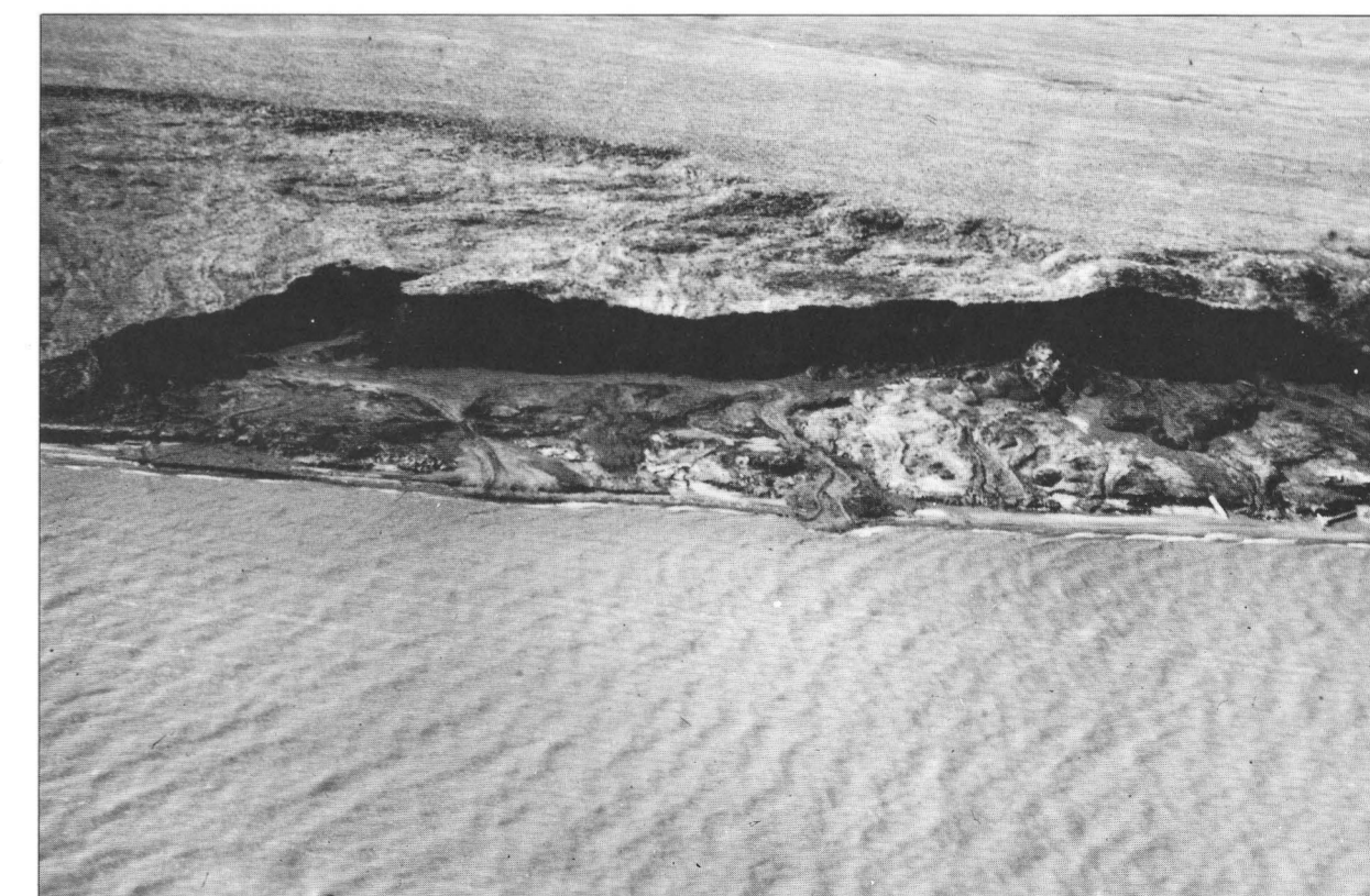
Aerial view of large retrogressive-thaw flow feature near Spring River, showing mudflow transport across the beach (8 August 1974). (GSC 202717G)
