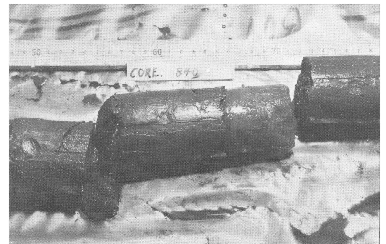
Sediment core containing lenses of freshwater ice. Core is broken at top of each ice lens; clay lies above the ice, and sand below it. Locality is in 36 m of water depth and lies 35 km north of Baillie Islands.
