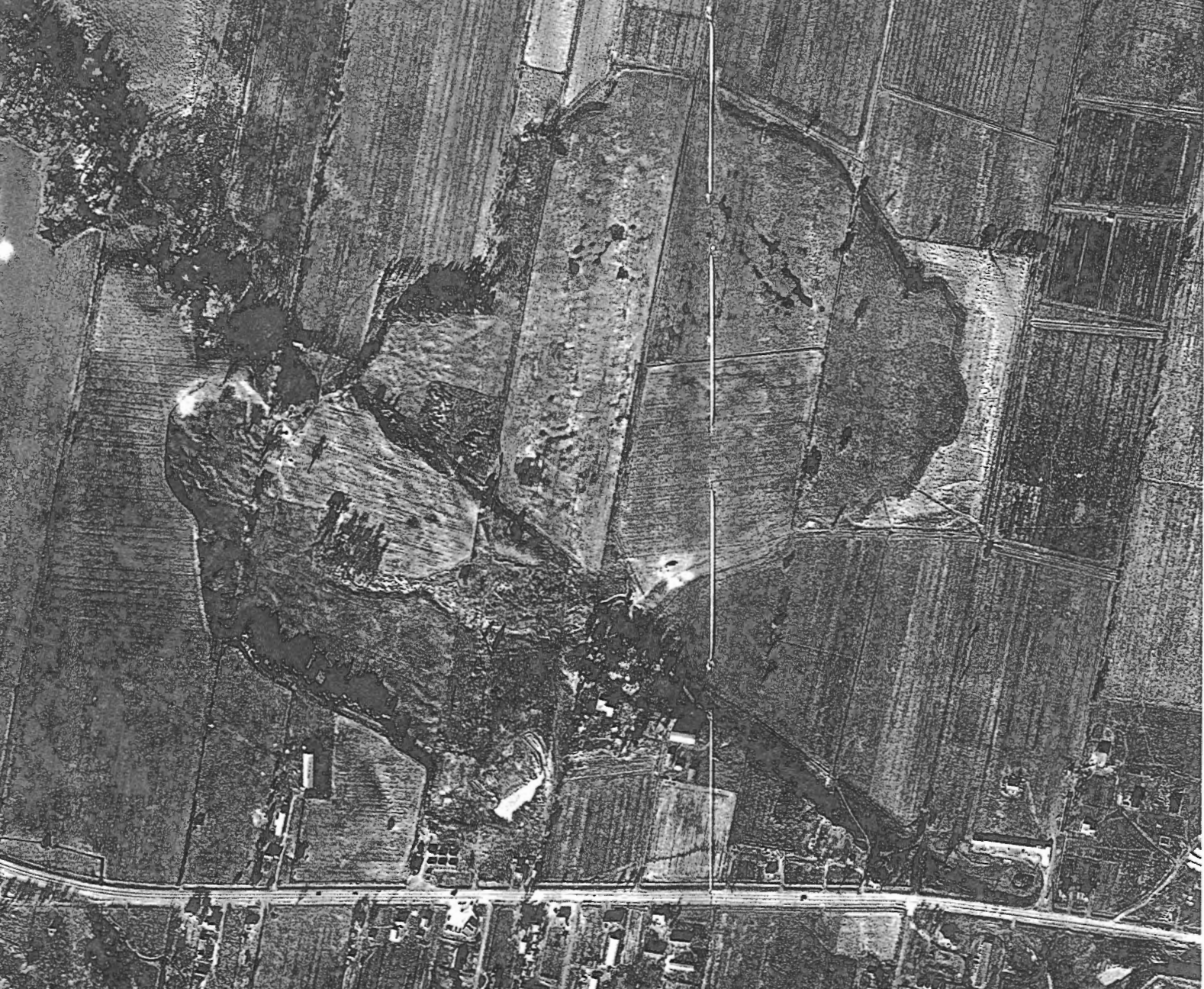
A beautiful example of a landslide in the clays of the Ottawa region at the east end of the city. The Montreal Road crosses the photograph near the lower margin and its intersection with the Queensway is at the lower right corner. The conspicuous terrace, out of which the clay has flowed out over the flats below, crosses the photograph diagonally. Note the pools and wet places in the toe of the landslide, showing that its surface is irregular by contrast with the very flat fields elsewhere.
