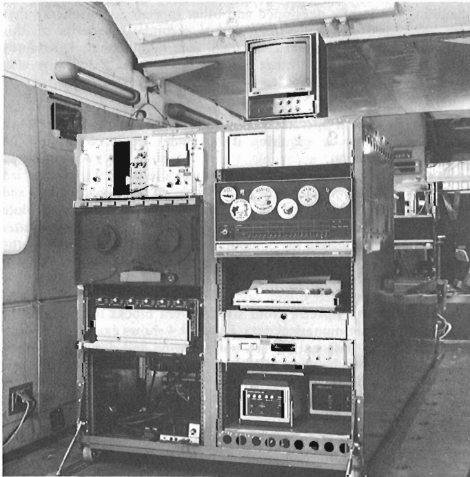
Figure 9-3. Complete gamma ray spectrometer in the Short Skyvan aircraft used for airborne research.
