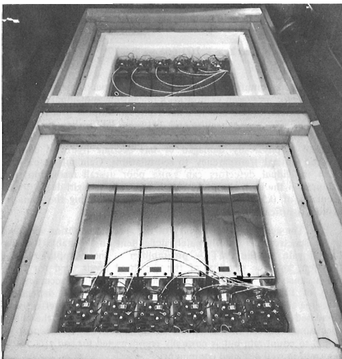
Figure 9-1. Twelve square prismatic NaI detectors packaged with preamplifiers in thermally insulated containers.
