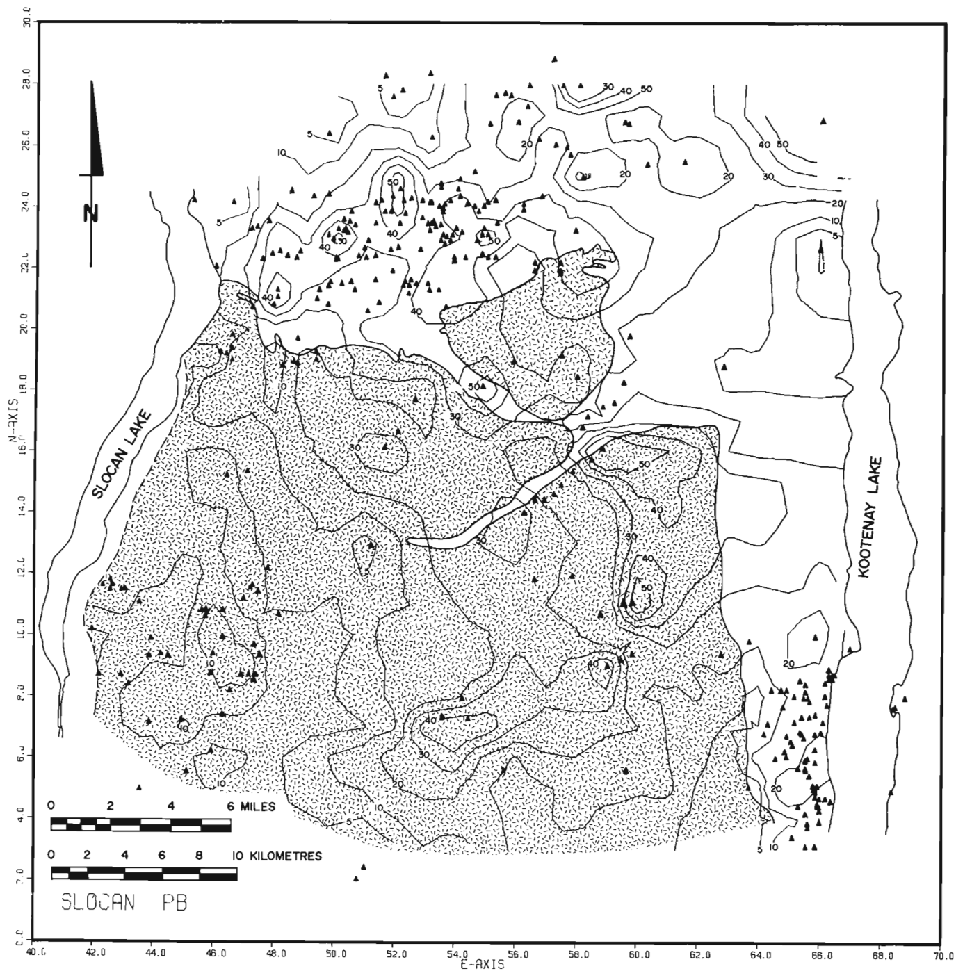
Figure 20.4. Machine-contoured plot of average Pb grades for about 340 vein deposits in and near the northern end of the Nelson batholith (patterned). Triangles are control points (deposits). Three principal concentrations of deposits (Slocan camp on the north, Slocan City camp on the southwest and Ainsworth camp on the southeast) stand out with centrally located pronounced Pb highs. Closed contours lacking control points on both sides or with very few control points are not considered significant.
