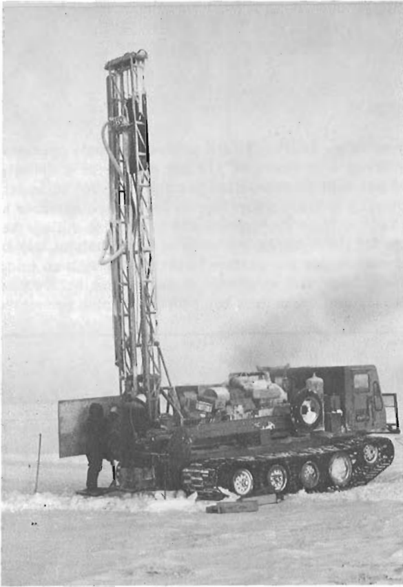
Figure 18.2. Flextrac Nodwell with Gardner-Denver air drill.
