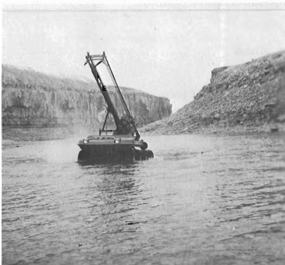
Figure 52.3. ATV-drill crossing a shallow river.
