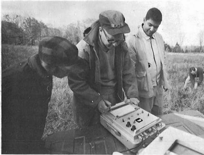
Figure 33.1. G. D. Hobson (centre) explaining the operation of the Hunttec FS-3 hammer seismograph to S. Samaniego (Philippines) and R. Bellety (Guyana), while C. M. H. Jennings (Botswana) strikes a steel plate with a sledgehammer to produce the seismic energy waves.
