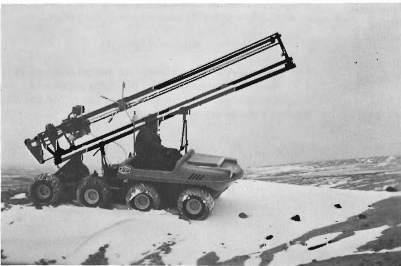
Figure 52.2. ATV-drill with retracted mast for travel.
