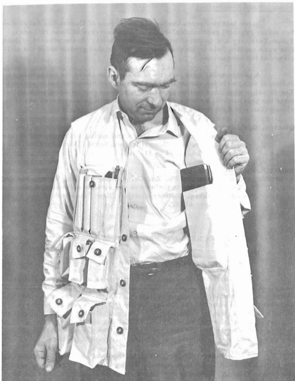
Figure 1. Geochemical field jacket, front view showing inside left hand pocket. G.S.C. Photo 113504-B.
