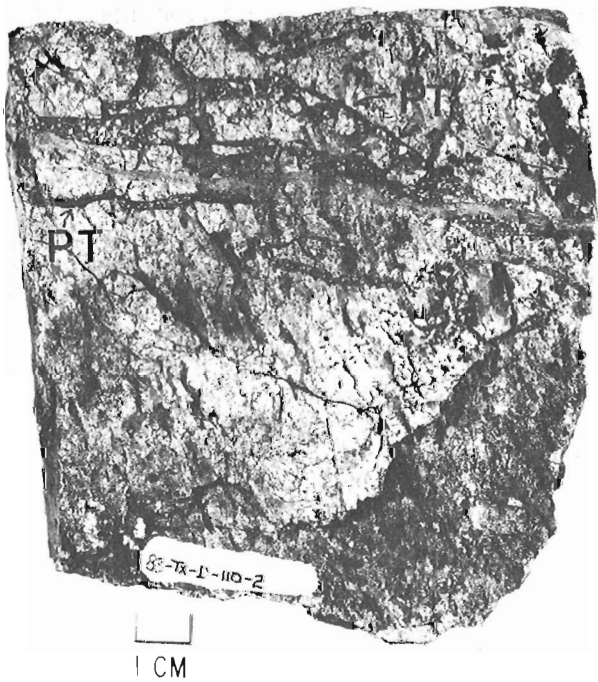
Figure 43.11. Breccia zones with pseudotachylite fractions cutting mylonitic layering; Chantrey Mylonite Zone. GSC 203308-V
