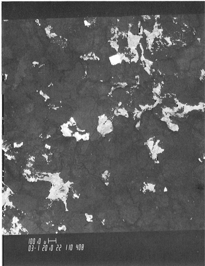
Figure 47.8. SEM photomicrograph (back scatter) of galena (light) in interstices of quartz grains (dark). Bright, square pyrite grain in upper centre.
