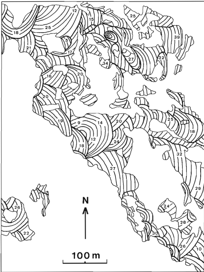
Figure 7.3. Objective field data map showing surface traces of crossbeds, lower bounding surfaces to sets, crossbed inclinations and areas of no outcrop. For detailed location see inset accompanying cross-section.
