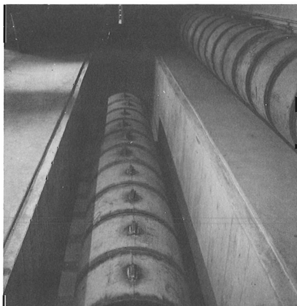
Figure 3. The multiple-zone horizontal model borehole in its below-ground tank, located in the Borehole Geophysics Laboratory at Aberdeen Street, Ottawa. (GSC 204145-B)
