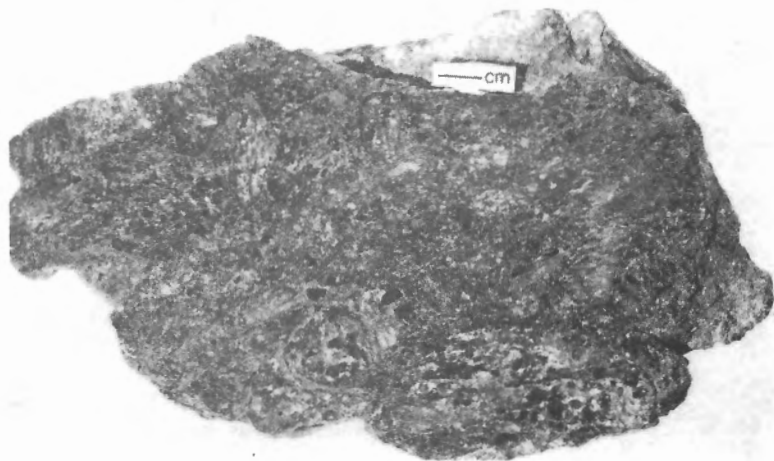
A. Photograph of mineralized uranium-copper bearing polymictic South Channel conglomerate, occurrence 8. (GSC 203345-H)
