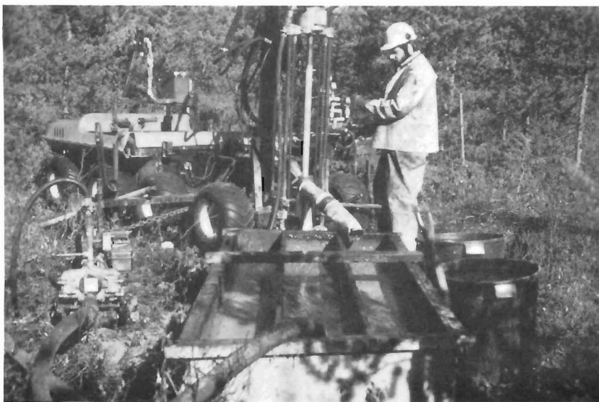
Figure 9.4. Coring with ATV-drill using an organic drilling fluid (Revert) recirculated by a light-weight mud pump. 203506-H.
