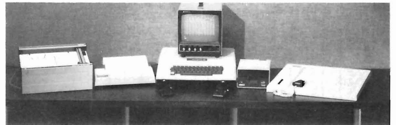
Figure 18.2. Apple II computer system with printer, plotter and digitizer.
