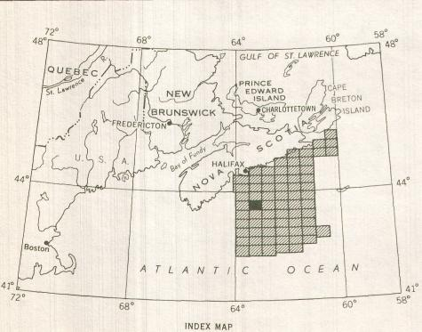
The ship magnetometer survey was conducted between May and Oct. 1962, using a direct-reading proton free-precession magnetometer. The ship's position was controlled by Nova Scotia Decca Chain 7 The survey and subsequent compilation were carried out by personnel from the Geophysics Division, Geological Survey of Canada. Drafting by Spartan Air Services Ltd.
