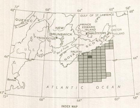
The ship magnetometer survey was conducted between May and June 1962, using a direct-reading proton free-precession magnetometer. The ship's position was controlled by Nova Scotia Decca Chain 7 The survey and subsequent compilation were carried out by personnel from the Geophysics Division, Geological Survey of Canada, Drafting by Spartan Air Services Ltd.
