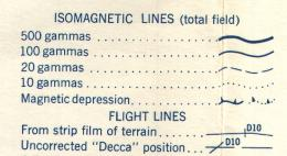
Magnetic Survey, May, 1958, by Geophysics Division, Geological Survey of Canada, Department of Mines and Technical Surveys. No correction has been made for regional variation; this increases at the rate of 6.1 gammas per mile from east to west and 3.5 gammas per mile from south to
