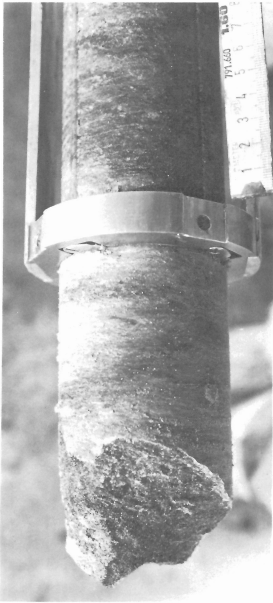
Figure 3. Detail of the core retriever and a section of core from 'Moraine pond' at Cape Herschel. Note the score marks made by the teeth as the retriever was pushed down over the core. May 19, 1981. GSC 203670-P
