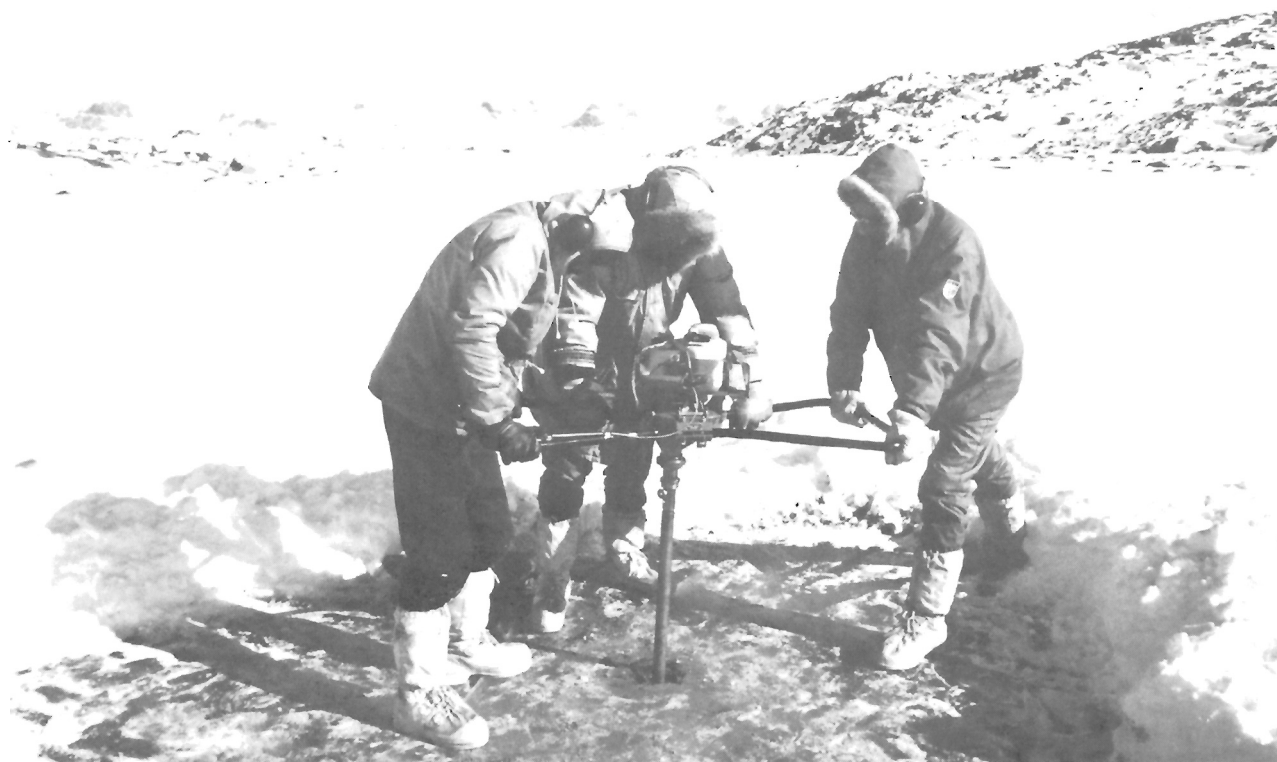
Figure 2. Coring underway with the Stihl motor unit at 'Willow Pond', north side of Cape Herschel peninsula. An 84 cm-long core was collected at this site, 8 m a.s.l. Pim Island is in the distance. May 25, 1981. GSC 203670-0
