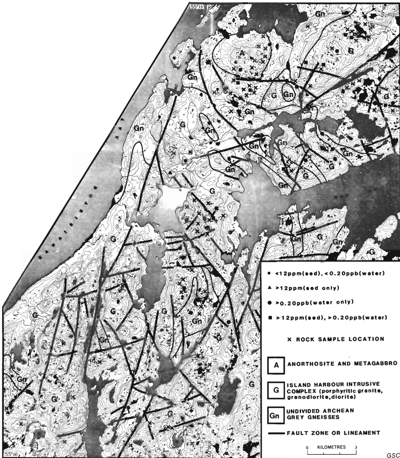
Figure 2.4. Generalized geology of Island Harbour Intrusive Complex (I. Ermanovics, personal communication), rock sample locations and distribution of uranium in lake waters and sediments. Regional threshold values for U in waters and sediments are 0.20 ppb and 12 ppm respectively.
