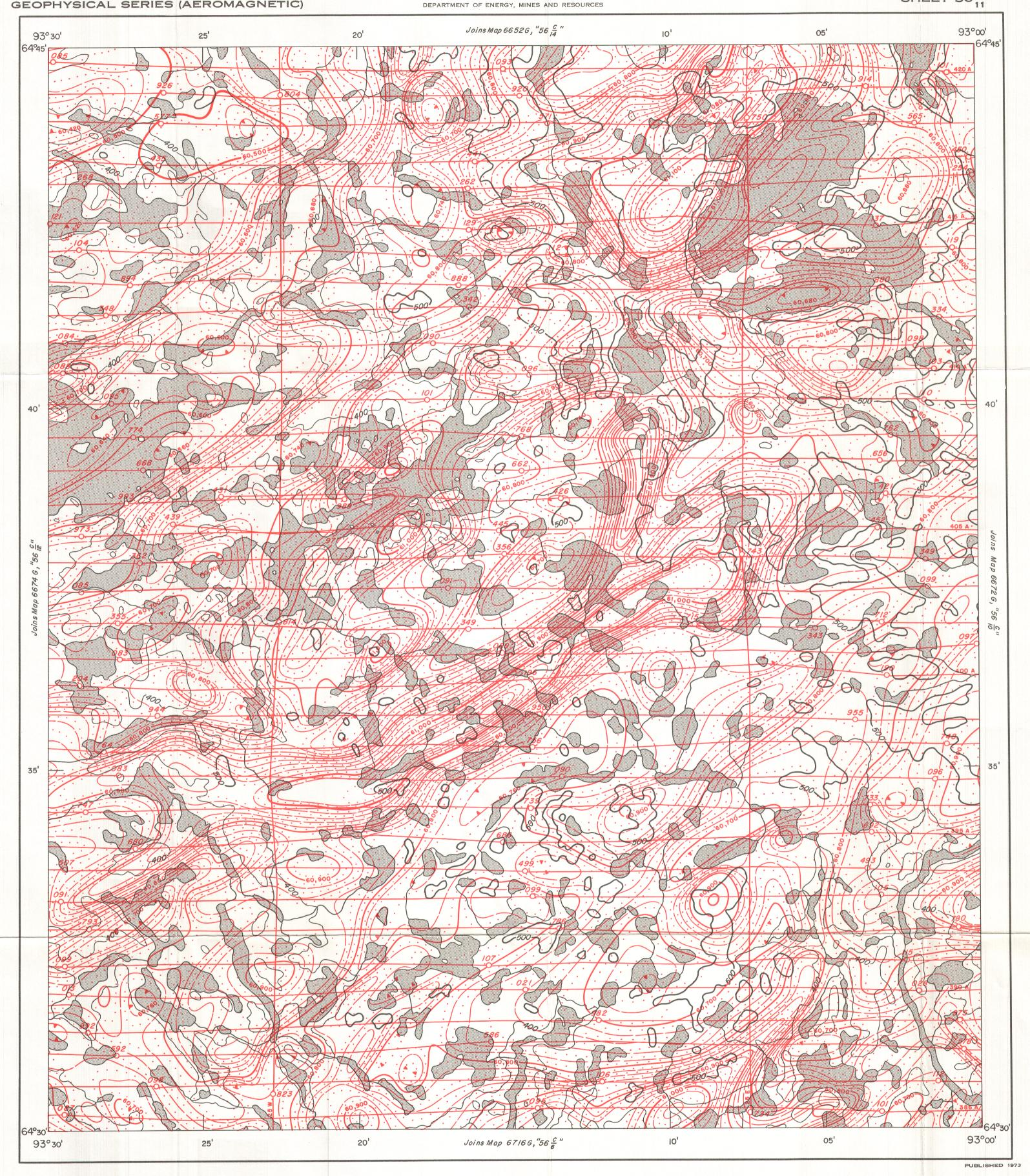
ISOMAGNETIC LINES (absolute total field) 500 gammas.... 100 gammas..... 20 gammas..... 10 gammas..... Magnetic depression.....
