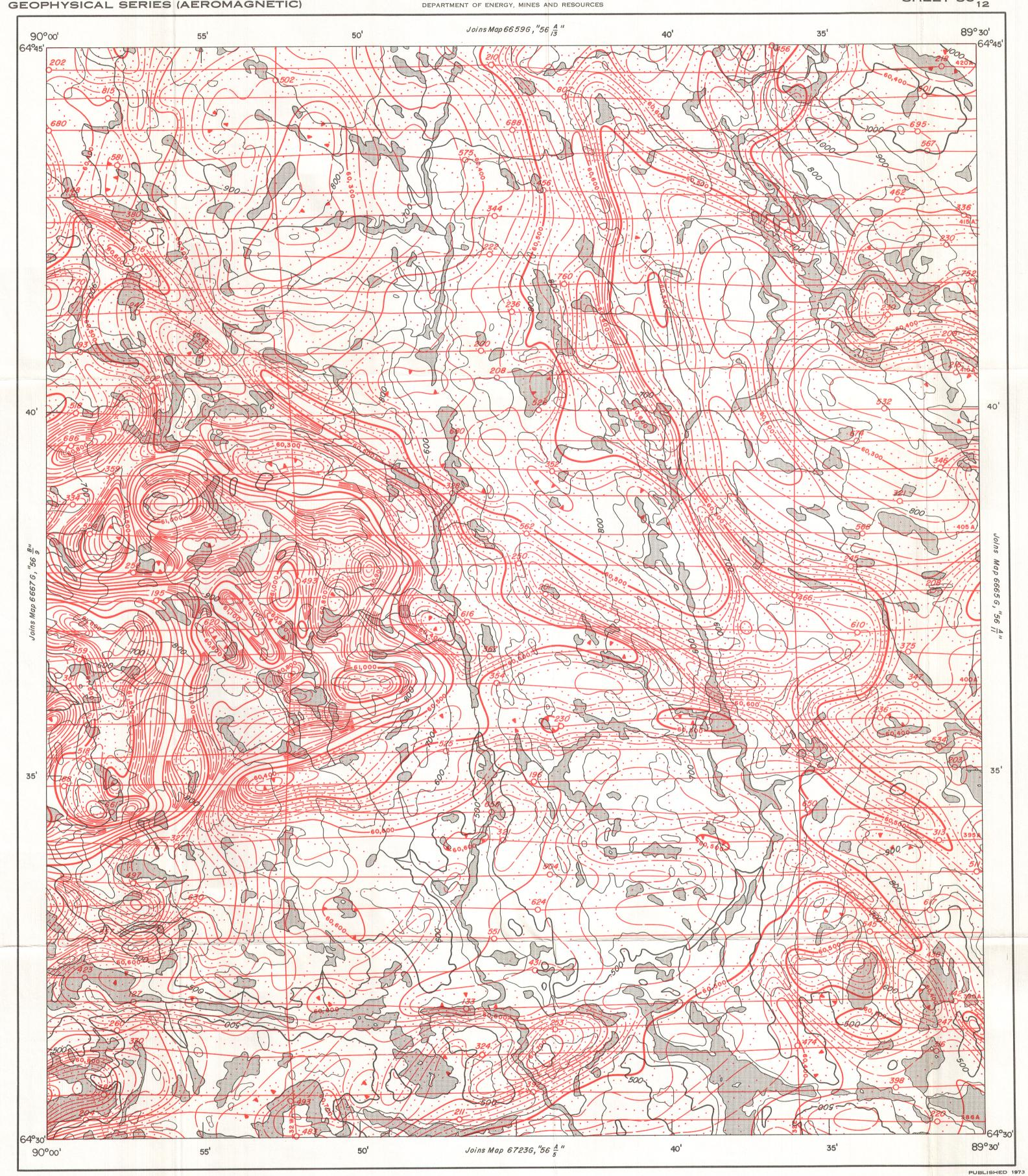
ISOMAGNETIC LINES (absolute total field) 500 gammas..... 100 gammas.... 20 gammas..... Flight lines.... Flight altitude 1000 feet above ground level
