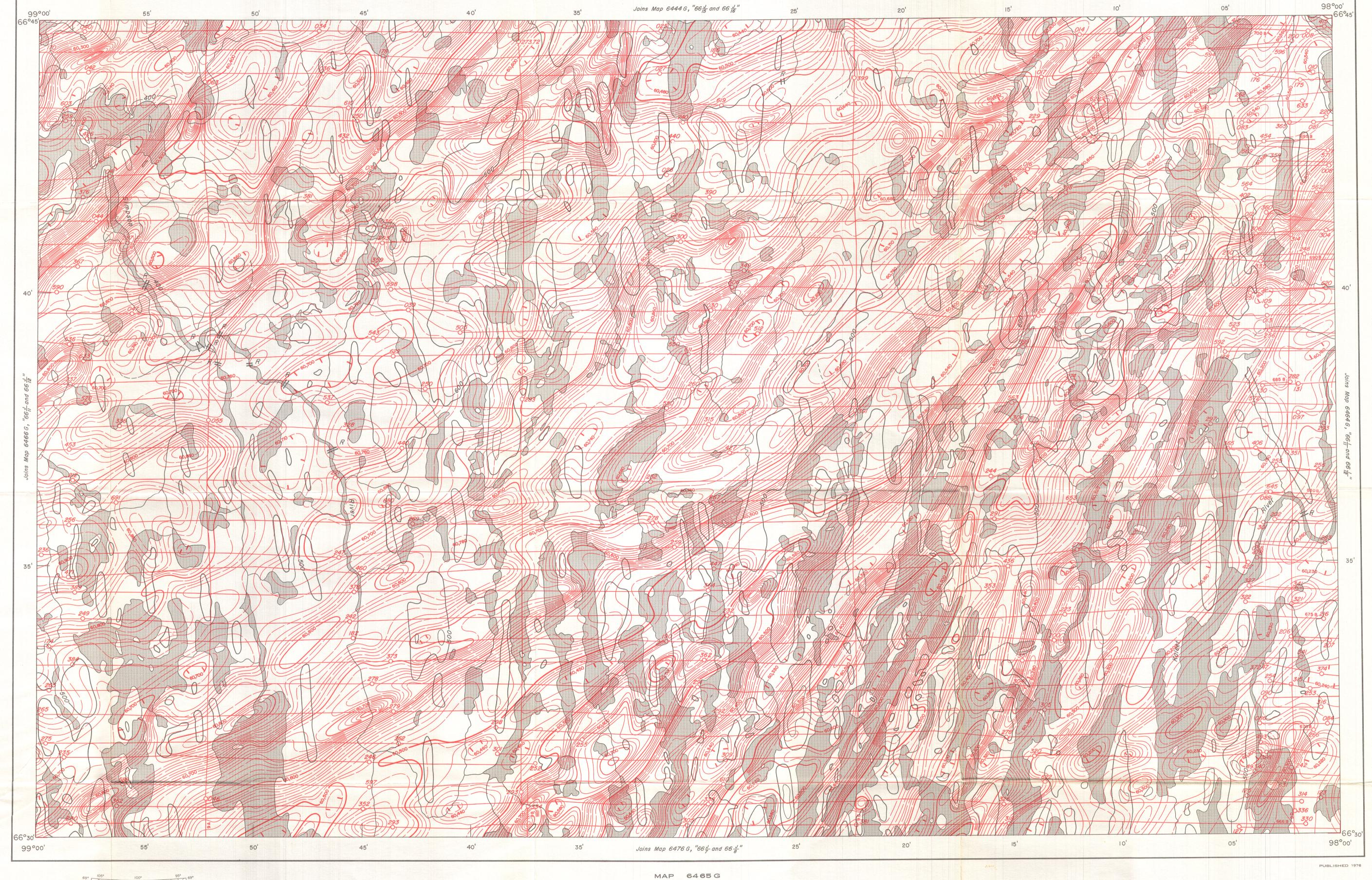
ISOMAGNETIC LINES (absolute total field) Flight altitude 1000 feet above ground level
