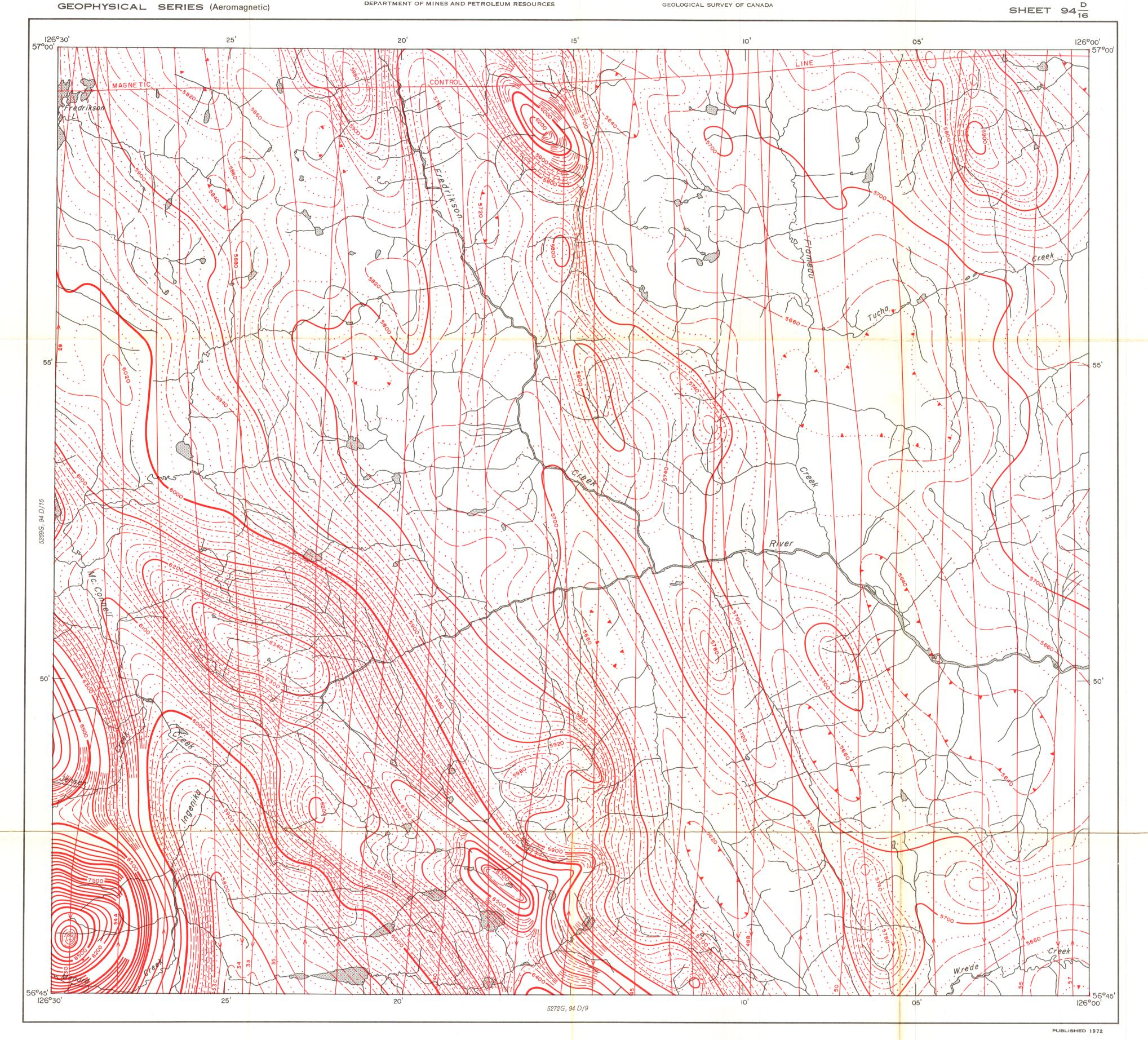
isomagnetic lines 500 gammas.... 100 gammas.... 20 gammas.... 10 gammas..... Flight lines.... Flight altitude 8500 feet above sea level
