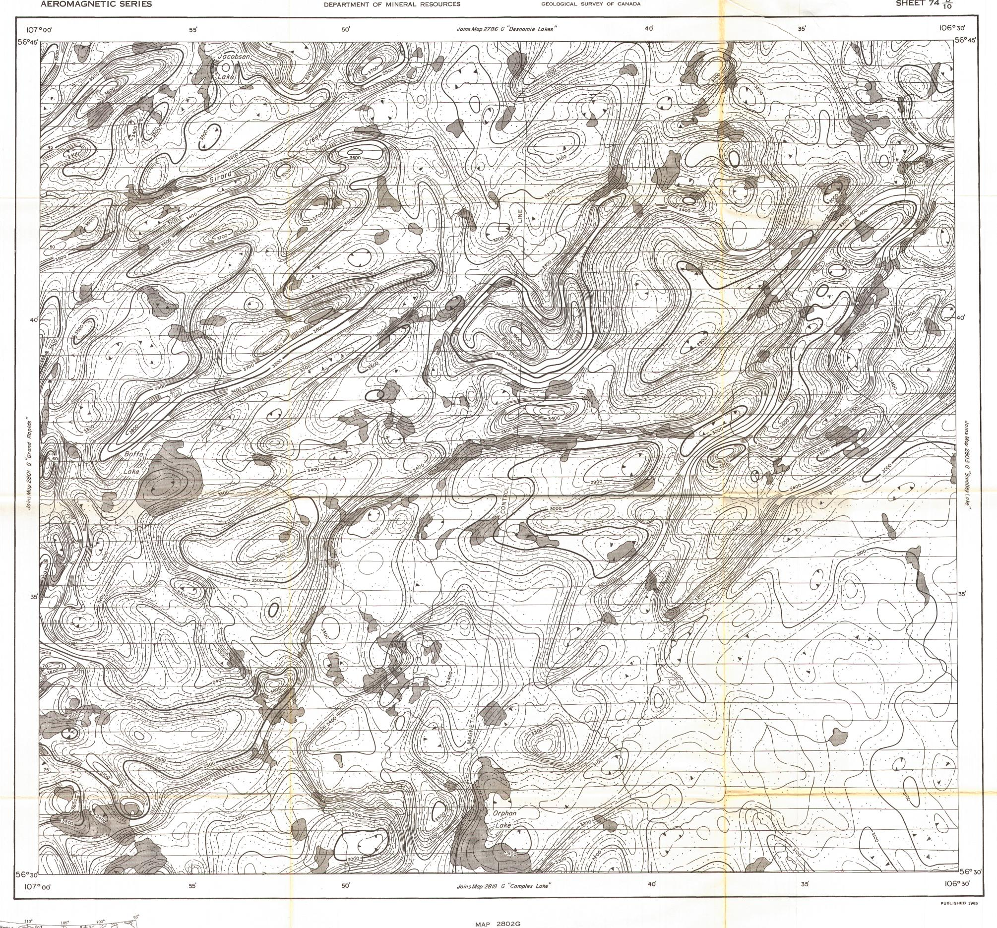
ISOMAGNETIC LINES (total field) 500 gammas. 20 gammas . . . . . . . 10 gammas.. ....... Magnetic depression.....
