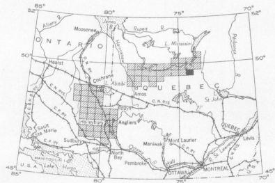
ISOMAGNETIC LINES (total field) 500 gammas... 100 gammas... Flight altitude 500 feet above ground level Flight line spacing (lines are not indicated) 1/4 mile (north, south)
