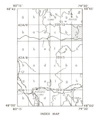
NOTE: Slight mismatches occur in some places between adjacent photomosaics used as base maps for this survey. These discontinuities were eliminated from the aeromagnetic data by adjustment and distribution routines in the automatic compilation system. As a result, some features on the printed mosaics may be displaced by up to 100 metres with respect to the aeromagnetic contours.
