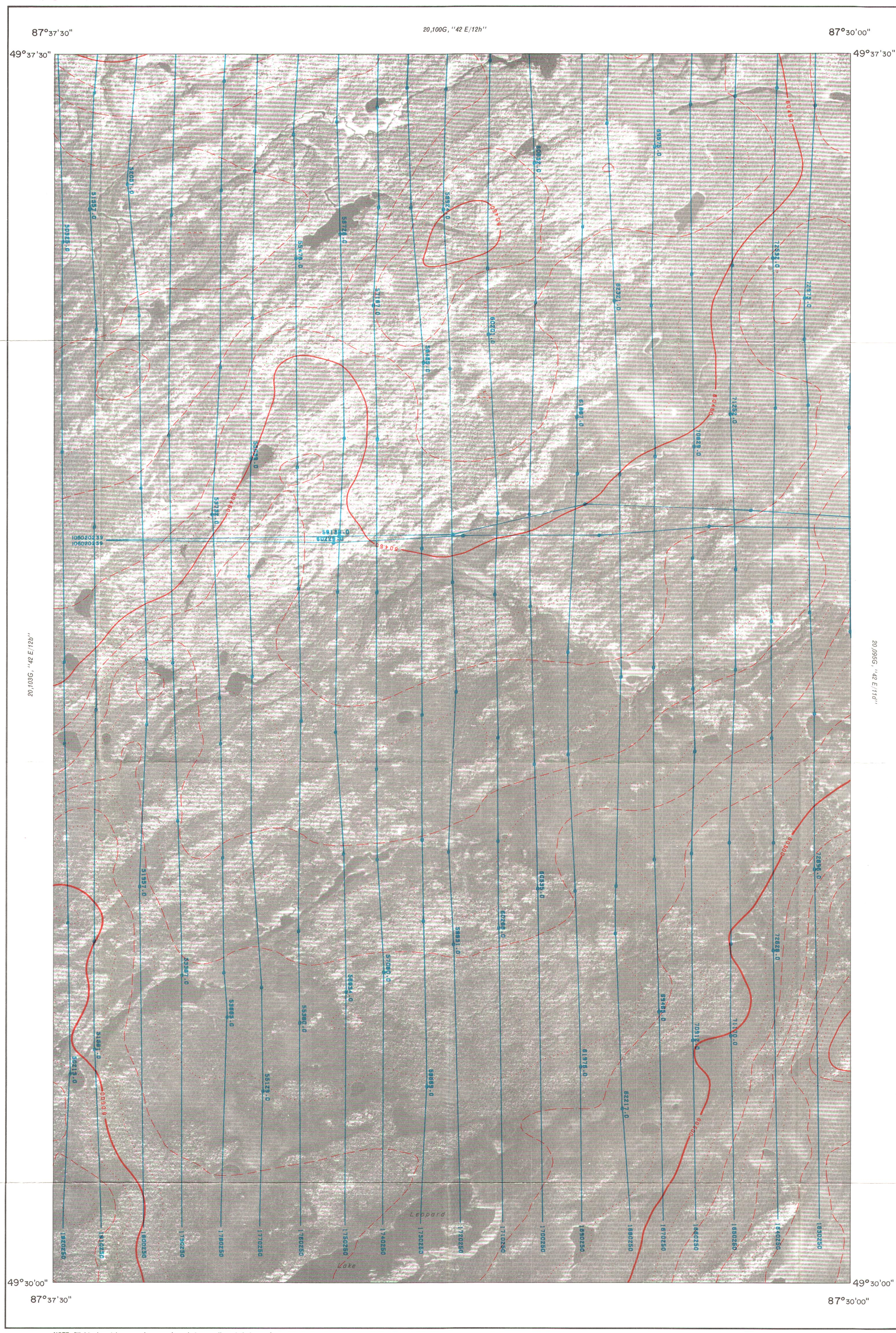
NOTE: Slight mismatches occur in some places between adjacent photomosaics used as base maps for this survey. These discontinuities were minimized from aeromagnetic data by using a digital data distribution routine in the automatic compilation system. As a result, some features on the printed mosaics may be displaced by up to 100 metres with respect to the aeromagnetic centres.
