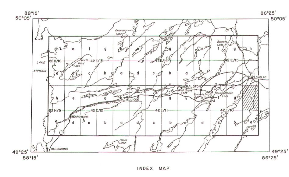
NOTE: Slight mismatches occur in some places between adjacent photomosaics used as base maps for this survey. These discontinuities were eliminated from the aeromagnetic data by adjustment and distribution routines in the automatic compilation system. As a result, some features on the primary map may be displaced by up to 100 metres with respect to the aeromagnetic contours.
