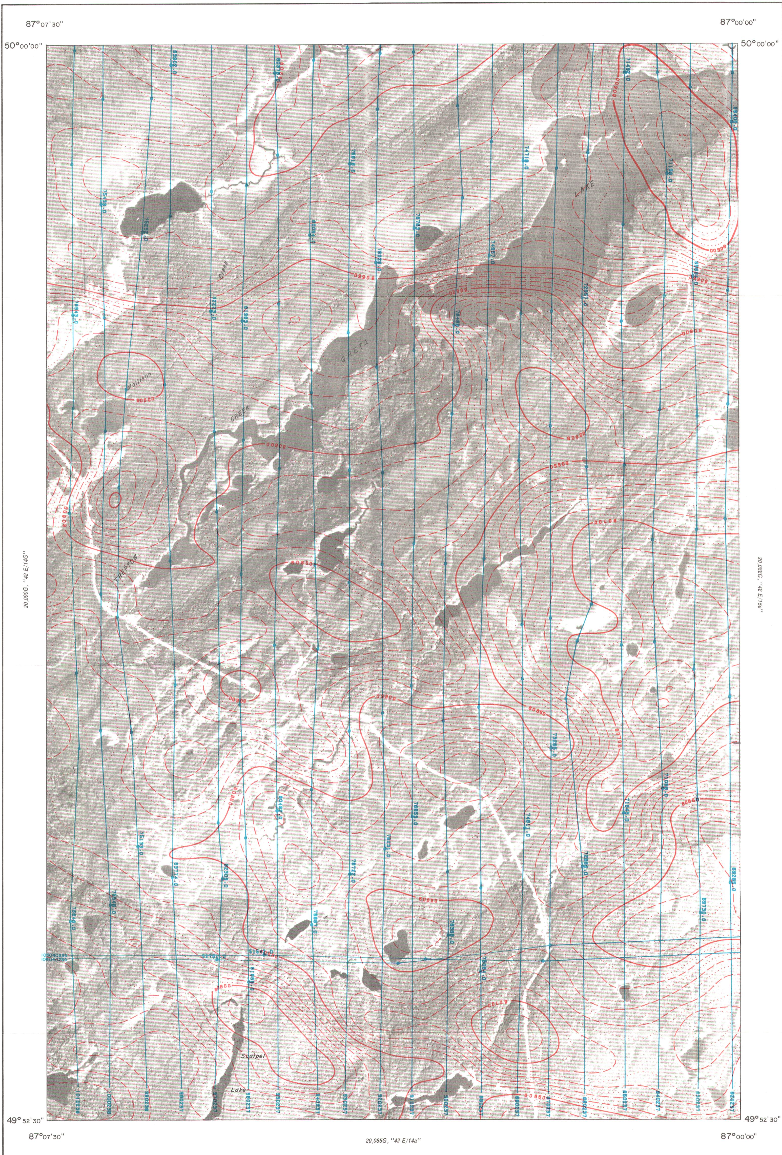
**NOTE:** Slight mismatches occur in some places between adjacent photomosaics used as base maps for this survey. These discontinuities were eliminated from the aeromagnetic data by adjustment and distribution routines in the automatic compilation system. As a result, some features on the printed mosaics may be displaced by up to 100 metres with respect to the aeromagnetic contours.
