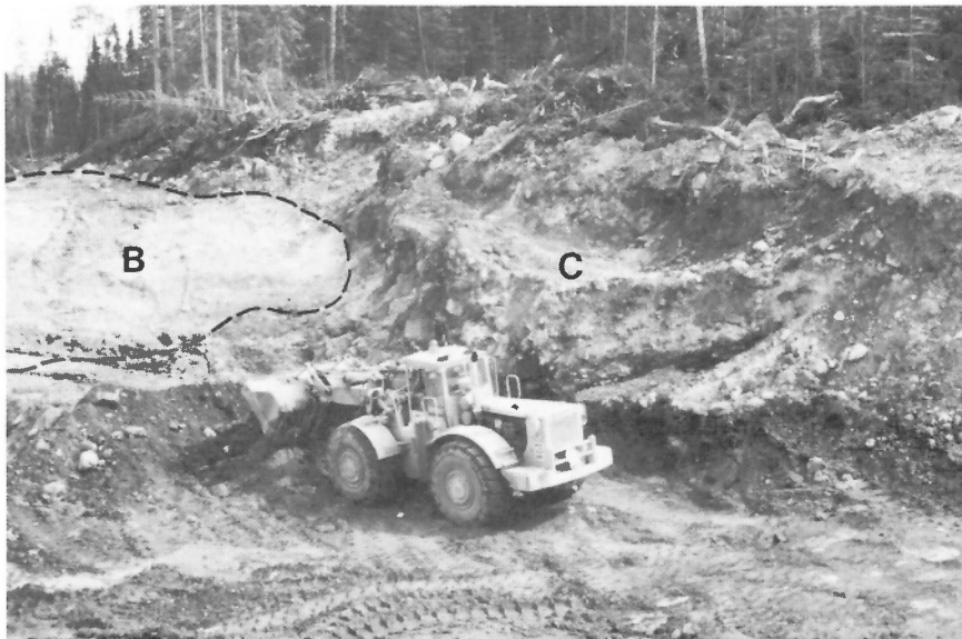
Figure 25. Mining till (unit C) from the up-ice end of the Icon train. Mound of unit B is light-toned area exposed by stripping in left background. Glacier that deposited unit C advanced away from the viewer. GSC 203518
