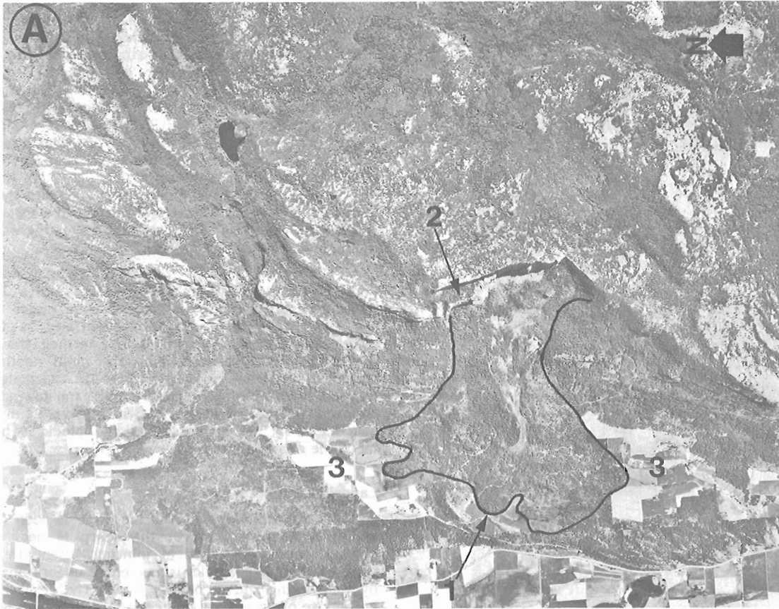
Figure 4. A. Aerial photograph of Enderby Cliffs; landslide is outlined. (BC 5190-158) 1 = active flow lobe; 2 = North Block; 3 = glaciolacustrine deposits.
