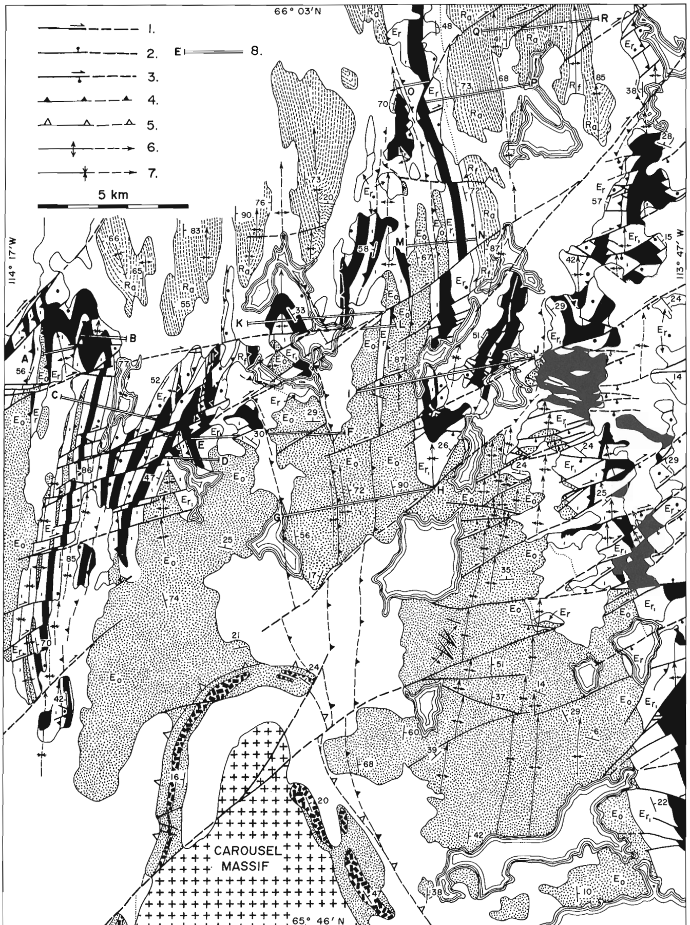
Figure 29.3. Geological map of Carousel Massif area, simplified from unpublished 1:50 000 maps, showing structural levels depicted on Figure 29.4. See Figure 29.2 for an explanation of stratigraphic symbols. 1. transcurrent fault; 2. normal fault; 3. oblique-slip fault; 4. thrust fault; 5. basal décollement; 6. plunging anticline; 7. plunging syncline; 8. projected structural level, Figure 29.4. 1-7 are inferred where dashed.
