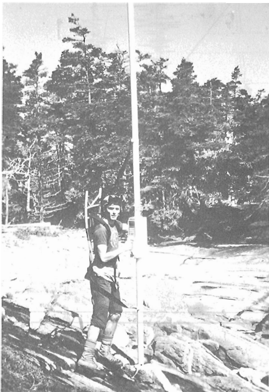
Figure 7.3. The EDA PPM-500 Vertical Magnetic Gradiometer in operation over an outcrop of the Goldenville Formation on Goose Island. GSC 203683-V.
