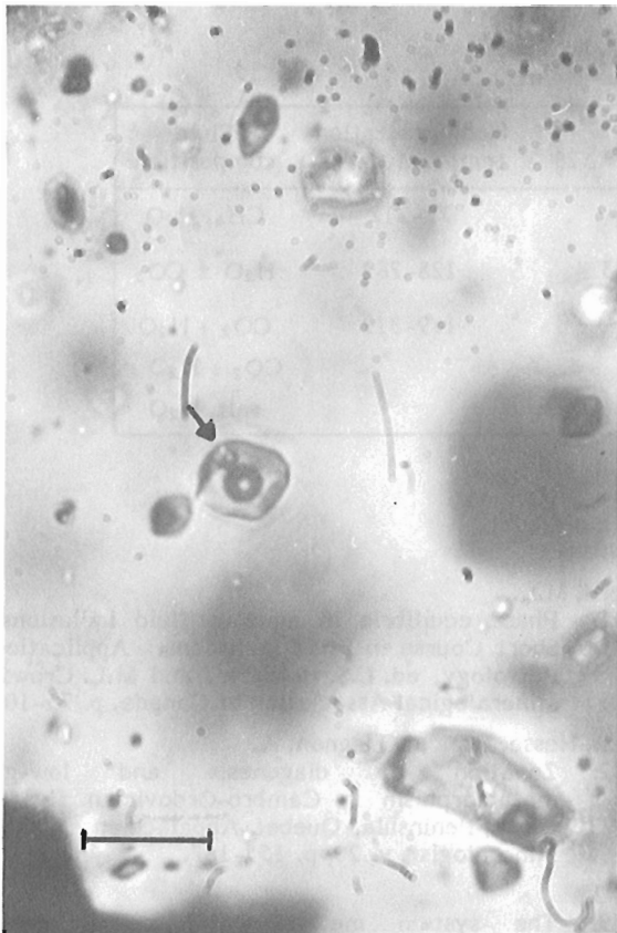
Figure 16.2c. Five-phase CO 2 -rich inclusion at centre with two salt crystals. Water is in outer rim, CO 2 vapour bubble at centre surrounded by liquid CO 2 . The salt crystals have not been identified. The other inclusions visible on this photomicrograph are water-rich. Sample no. CC-73. Scale bar is 40 microns.
