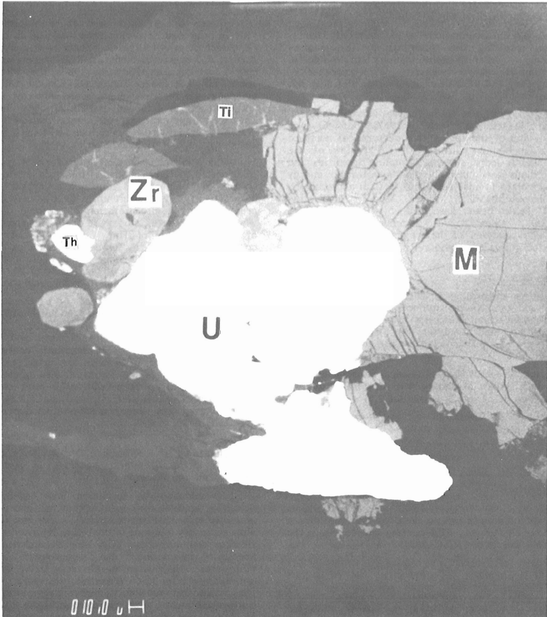
Figure 3.2. BEI of an association of radioactive ore minerals: uraninite (U) and uranothorite (Th), and of accessory minerals: magnetite (M), zircon (Zr) and titanite (Ti). The uraninite apparently replaces magnetite and zircon at the northern margin. Zircon has a mottled appearance and is intergrown with uranothorite which is enclosed in a prominent rim having disseminated specks of galena (white) and of radioactive and REE compounds (various shades of grey). Titanite grains are overgrown and traversed along fractures by U-bearing crusts (white). Magnetite is fractured as a result of radiation from the adjacent uraninite. Melanocratic ore, Madawaska mine (GSC 203577-S).
