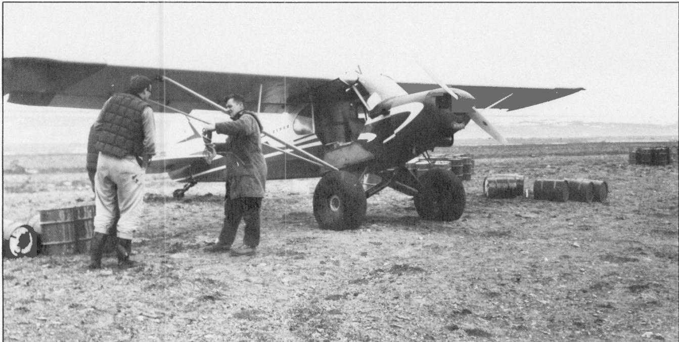
The Geological Survey pioneered the use of light aircraft equipped with low-pressure, balloon tires. The land surface in parts of the Arctic is relatively flat and in many places there are innumerable raised beaches. Both features allow landings to be made on unprepared sites. Note the 45 gallon gas drum in the cabin. This was used for long, staging flights from southern Canada.
