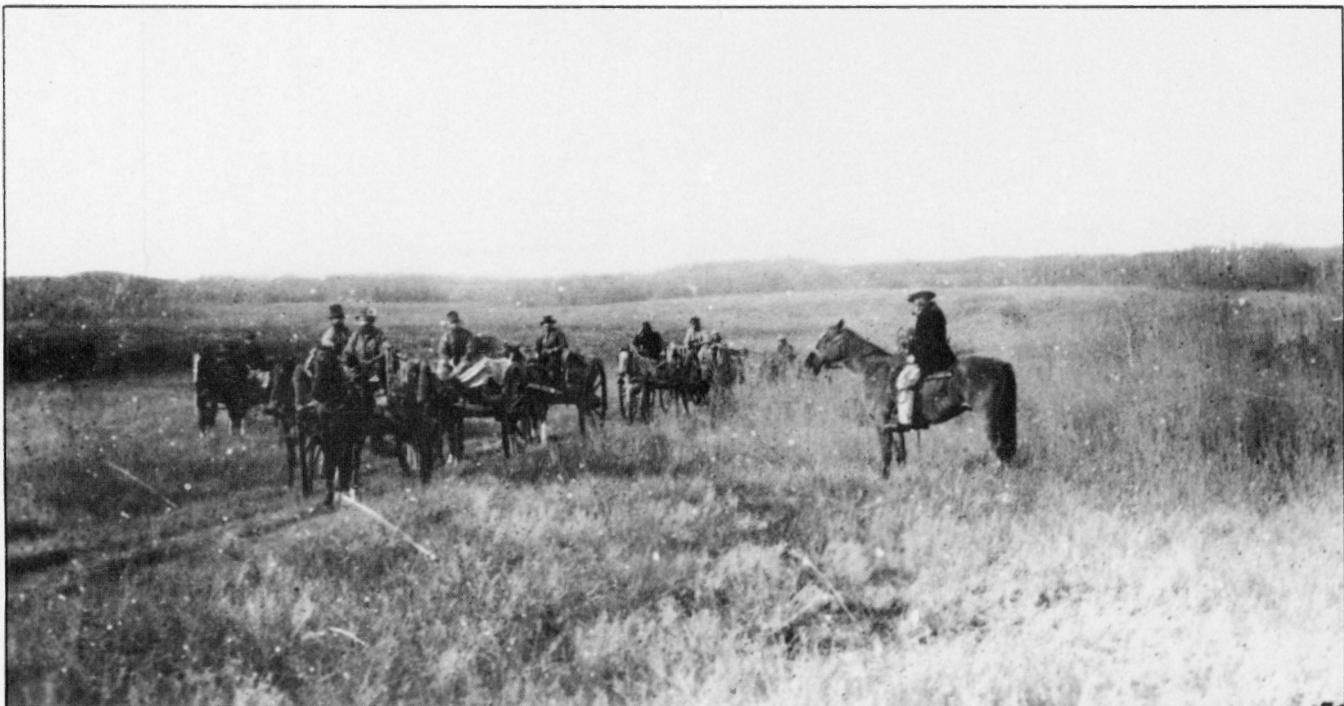
**Train of Red River carts, 1879.** Prior to the coming of the railways Red River carts were almost indispensable to prairie travellers. Constructed entirely of wood, they were easily repairable. Even when timber was not available the hide of a freshly killed buffalo wrapped around the broken ends would soon dry and tightly bind the pieces.
