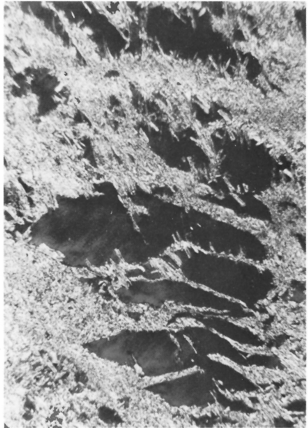
A. Fractured picotite. x 16 plain light. GSC 203173
