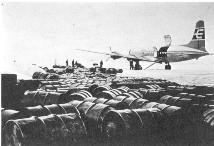
Figure 2. The DC-6 freighter aircraft unloading part of the 25,000 gallons of diesel fuel airlifted to Speers Lake, Northwest Territories, for the Muskox Drilling Project.
