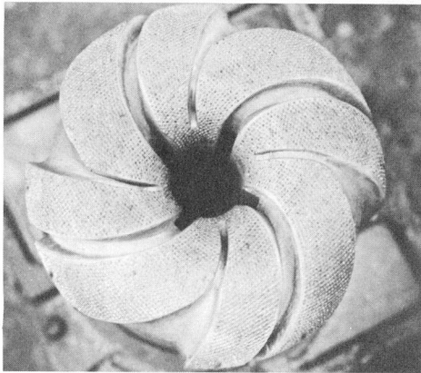
Figure 5. Three of the diamond bits used with the turbocorer. The thousands of diamonds in each bit penetrate about .002 inch per revolution. At 600 rpm this results in a rate of advance of about 5 1/2 feet per hour.
