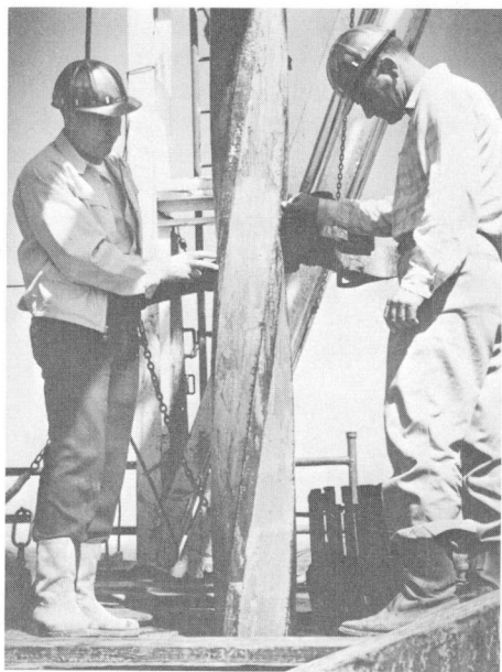
Figure 7. Square spiral outer core barrel which provides a high degree of stabilization was tested at Uvalde. The barrel is 1/16-inch under bit gauge and is 26 feet long. Stabilizers were run immediately above and below the barrel.
