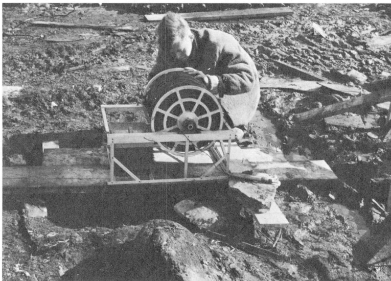
Figure 5. Portable temperature measuring equipment used for logging the Muskox North drill-hole.
