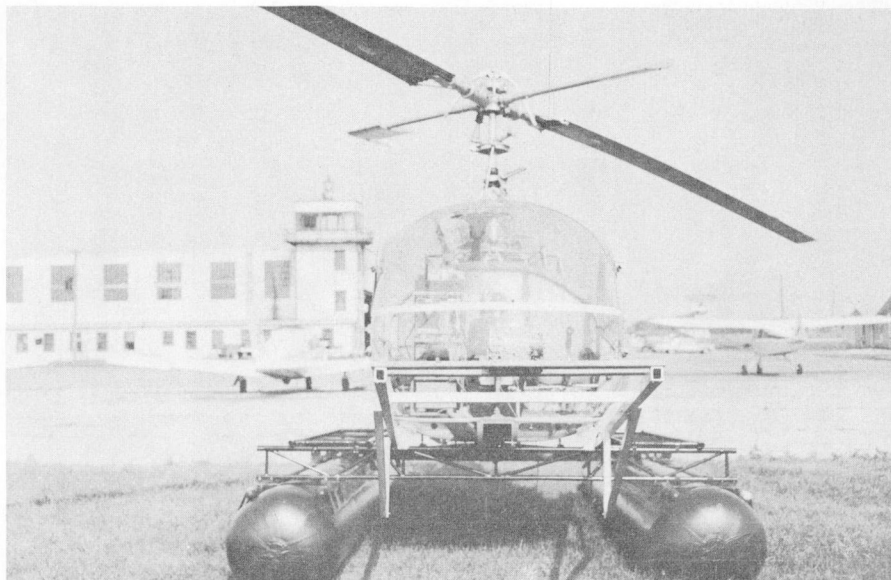
Plate 2. A front view of the helicopter showing the boom attached to the aircraft and the sensing head in the foreground
