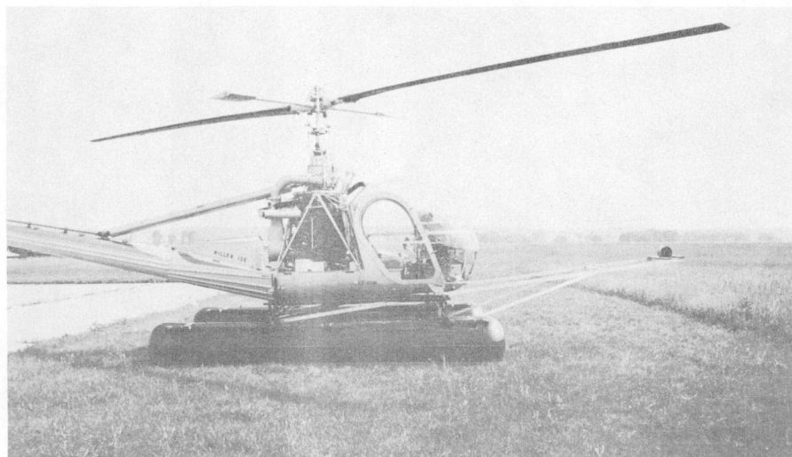
Plate 3. A side view of the Hiller 12E with the telemetering magnetometer equipment installed, ready for a survey flight
