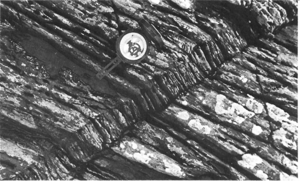
Plate 1A. Dextral kink band showing parallel kink planes marked by joints. (Knockinelder)
