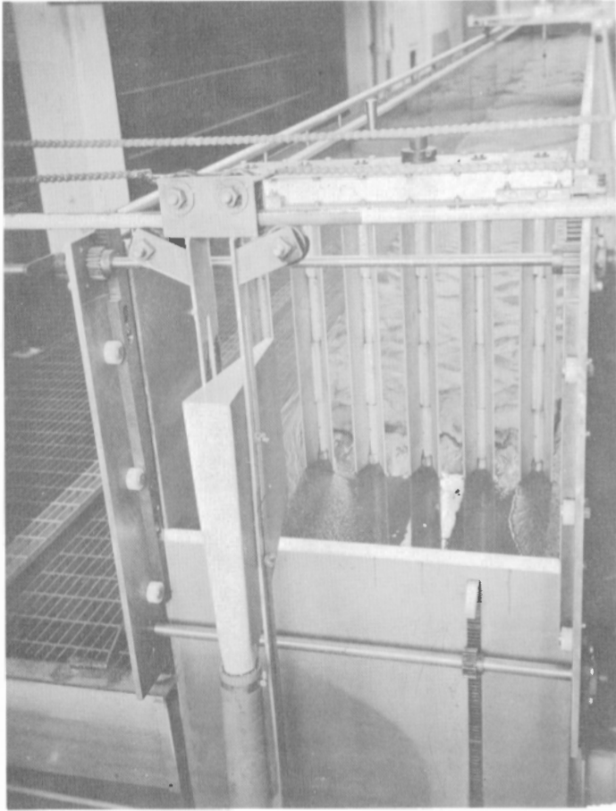
Figure 4. Vertically hinged louvered tailgate and total-load sampler. GSC photo 201625-I
