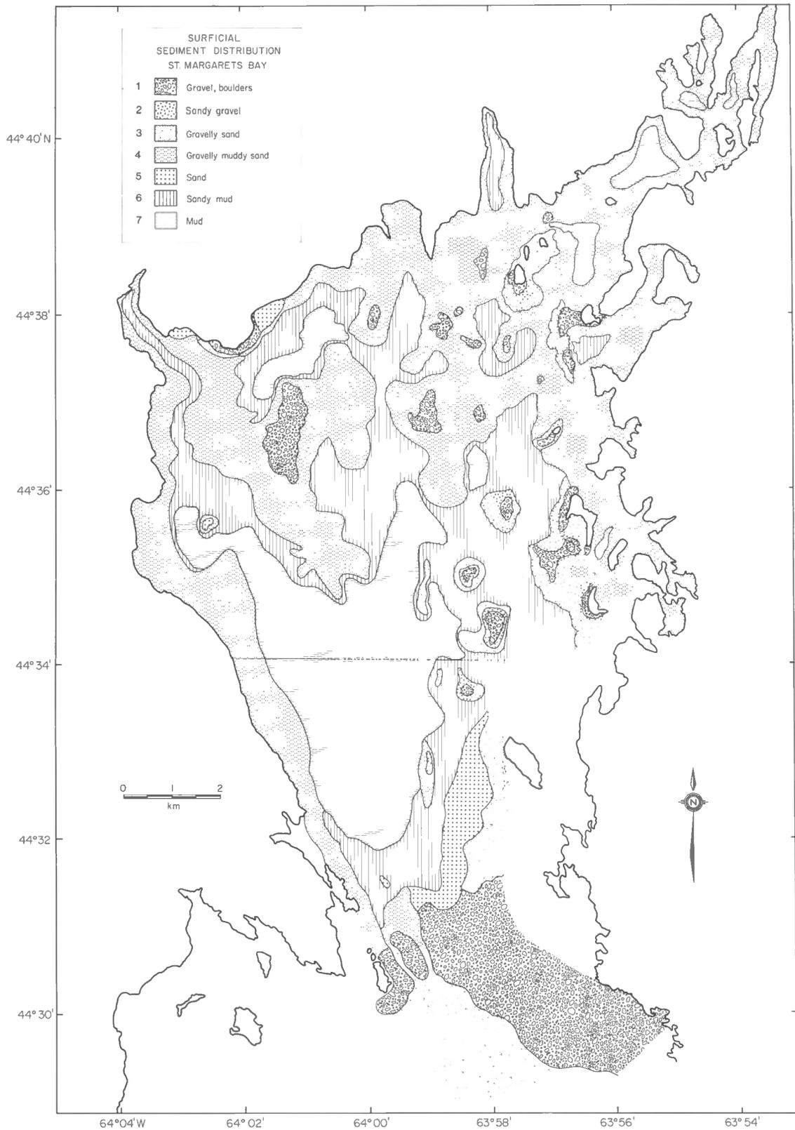
Figure 13. Distribution of surficial sediments in St. Margaret's Bay. Based on MS26B echo sounder profiles and surficial sediment samples.
