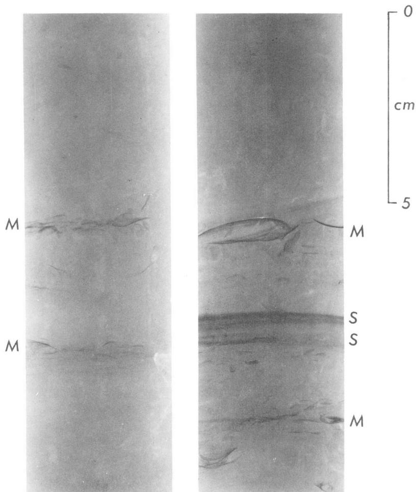
Figure 14. X-radiography of silty laminae in core 74-021-1.
