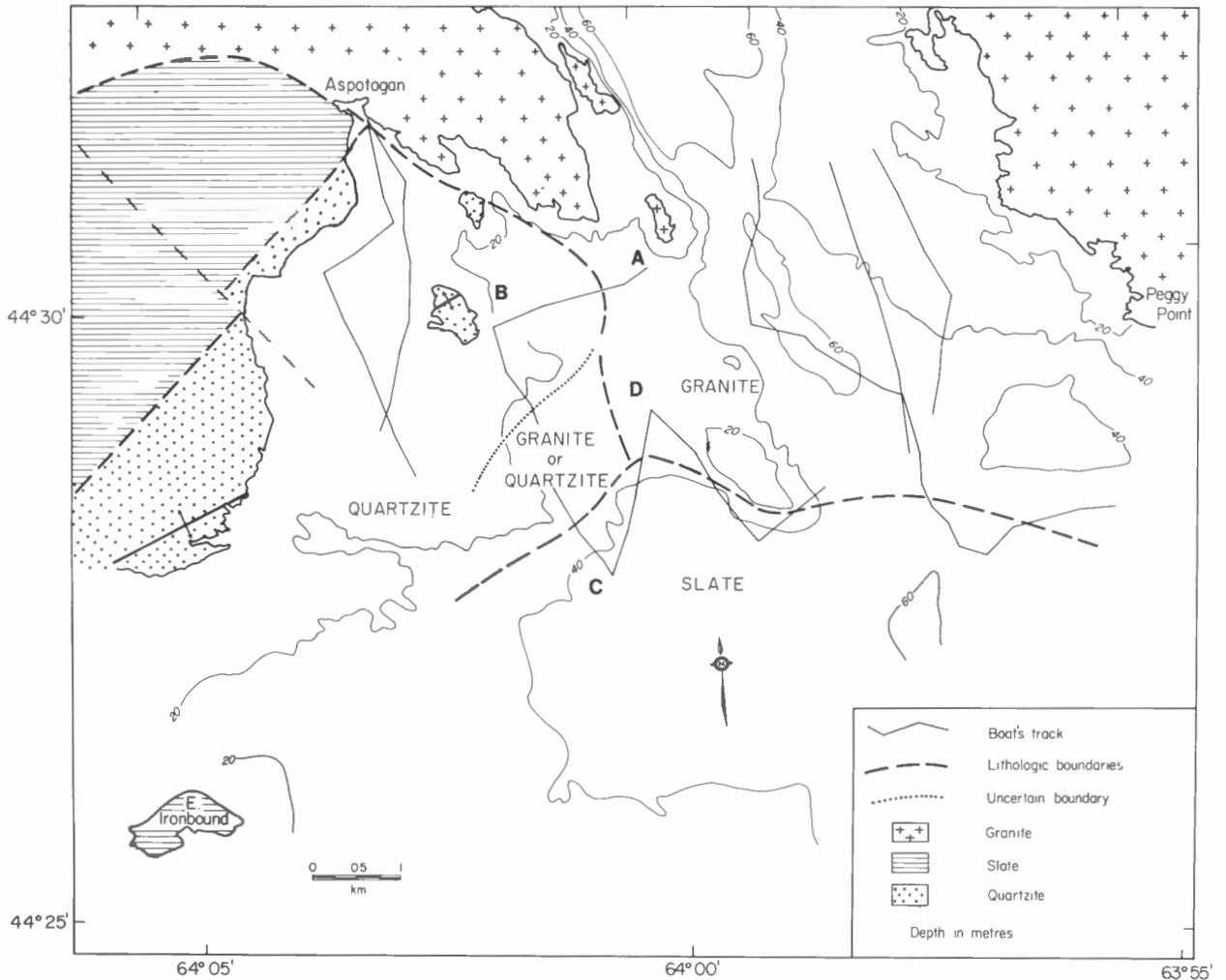
Figure 7. Inferred offshore geology south of Aspotogan, based on magnetometer profiles. Typical profiles shown in Figure 8. Land geology based on Sage (1954).
