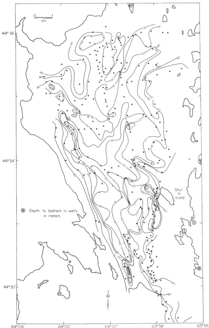
Figure 5. Map showing "depth" to bedrock, contoured in 2-way reflection time in milliseconds. Dots represent data points.
