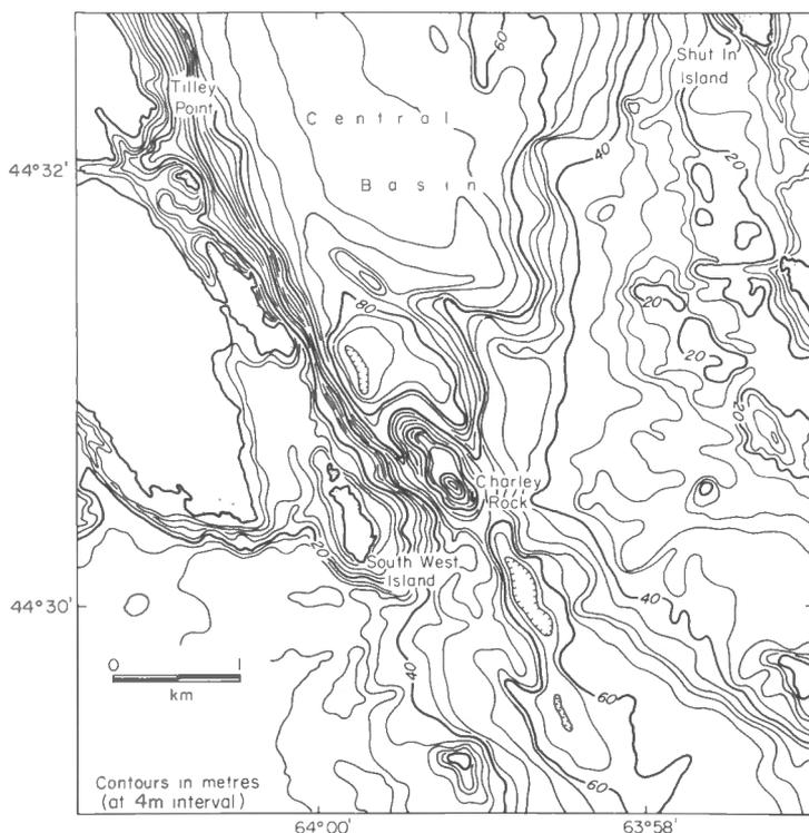
Figure 3. Detailed bathymetric map of entrance to St. Margaret's Bay. Contours at 4-m intervals based on fathom soundings on Hydrographic Service field sheets.
