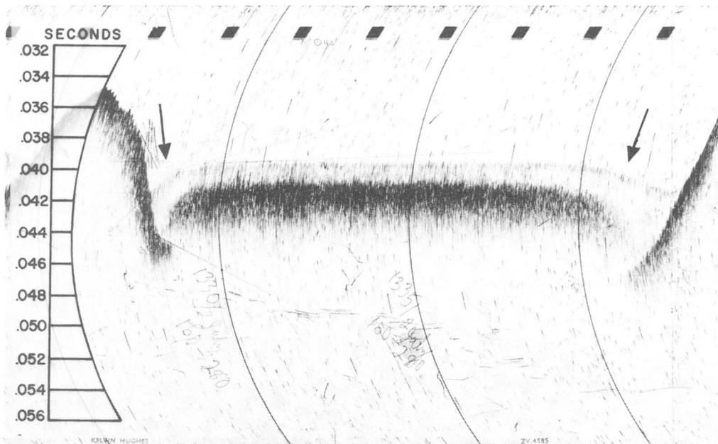
Figure 15. MS26B record showing "two metre" reflector (between arrows).
