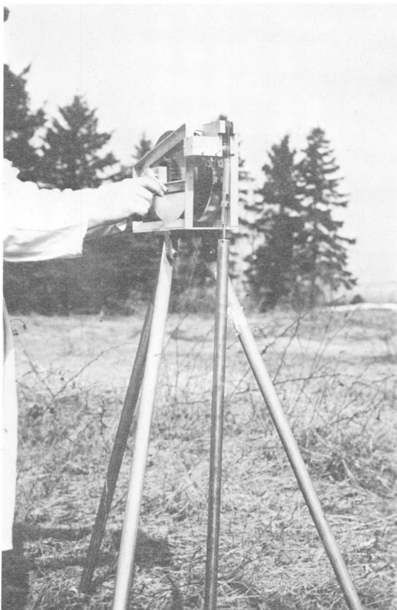
Figure 3. Small diameter drill hole water sampler and winch assembly.
