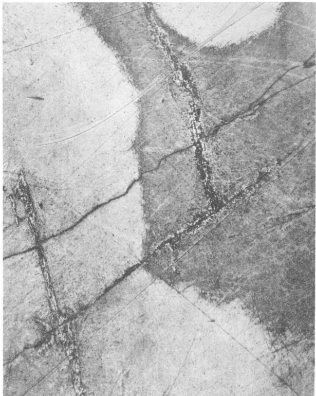
Figure 3. Etched polished surfaces treated with magnetite colloid showing co-existence of a magnetic ( \text{Fe}_7\text{S}_8 ) and a non-magnetic ( \text{Fe}_9\text{S}_{10} ) pyrrhotite type.
