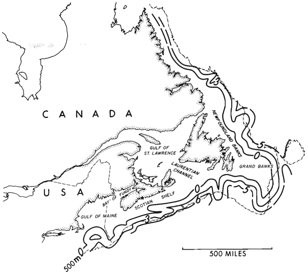
Figure 10. Velocity layer 2, Compressional Velocities 7,300-11,200 ft/sec (2.2-3.4 km/sec). Isopach Interval in thousands of feet.
