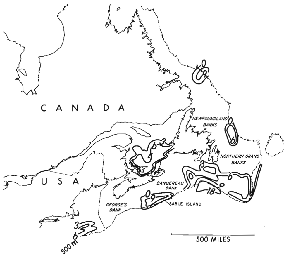
Figure 11. Velocity Layer 3, Compressional Velocities 10,500-14,800 ft/sec (3.2-4.5 km/sec). Isopach Interval in thousands of feet.
