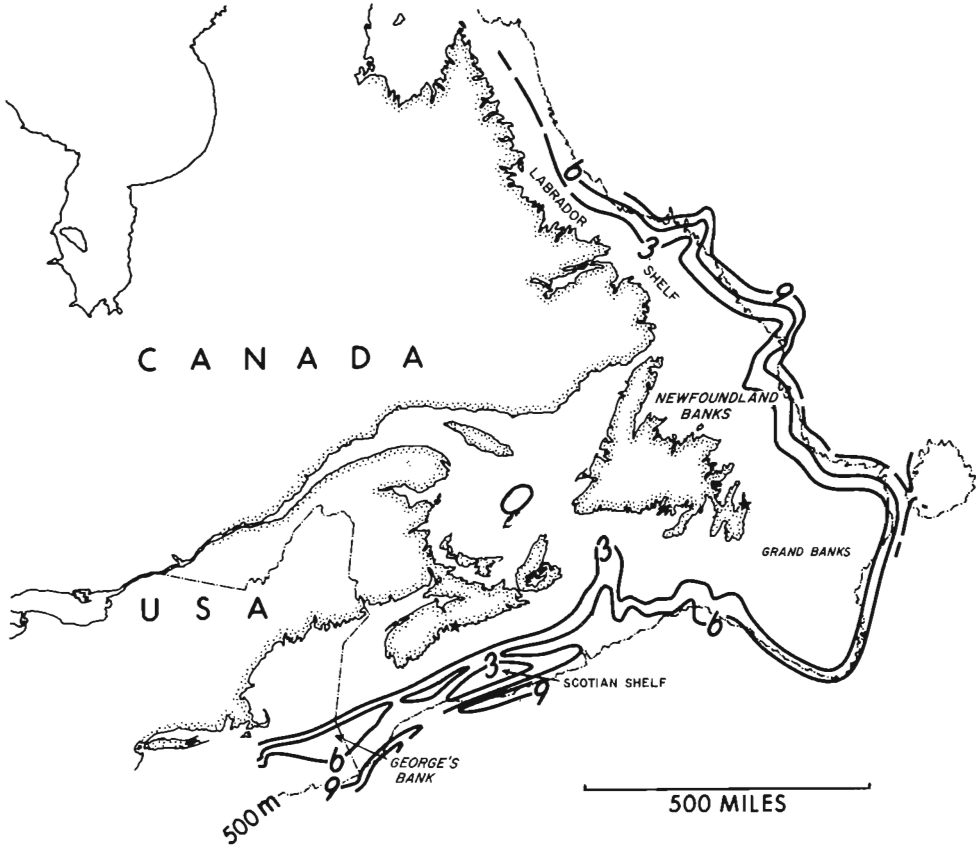
Figure 9. Velocity layer 1, Compressional Velocities 5900-7200 ft/sec (1.8-2.2 km/sec). Isopach Interval in thousands of feet.
