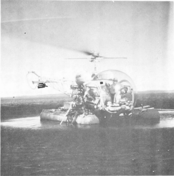
Plate 3. Sampling near shore lake sediment from the Bell G4A helicopter. GSC Photo 202132C.
