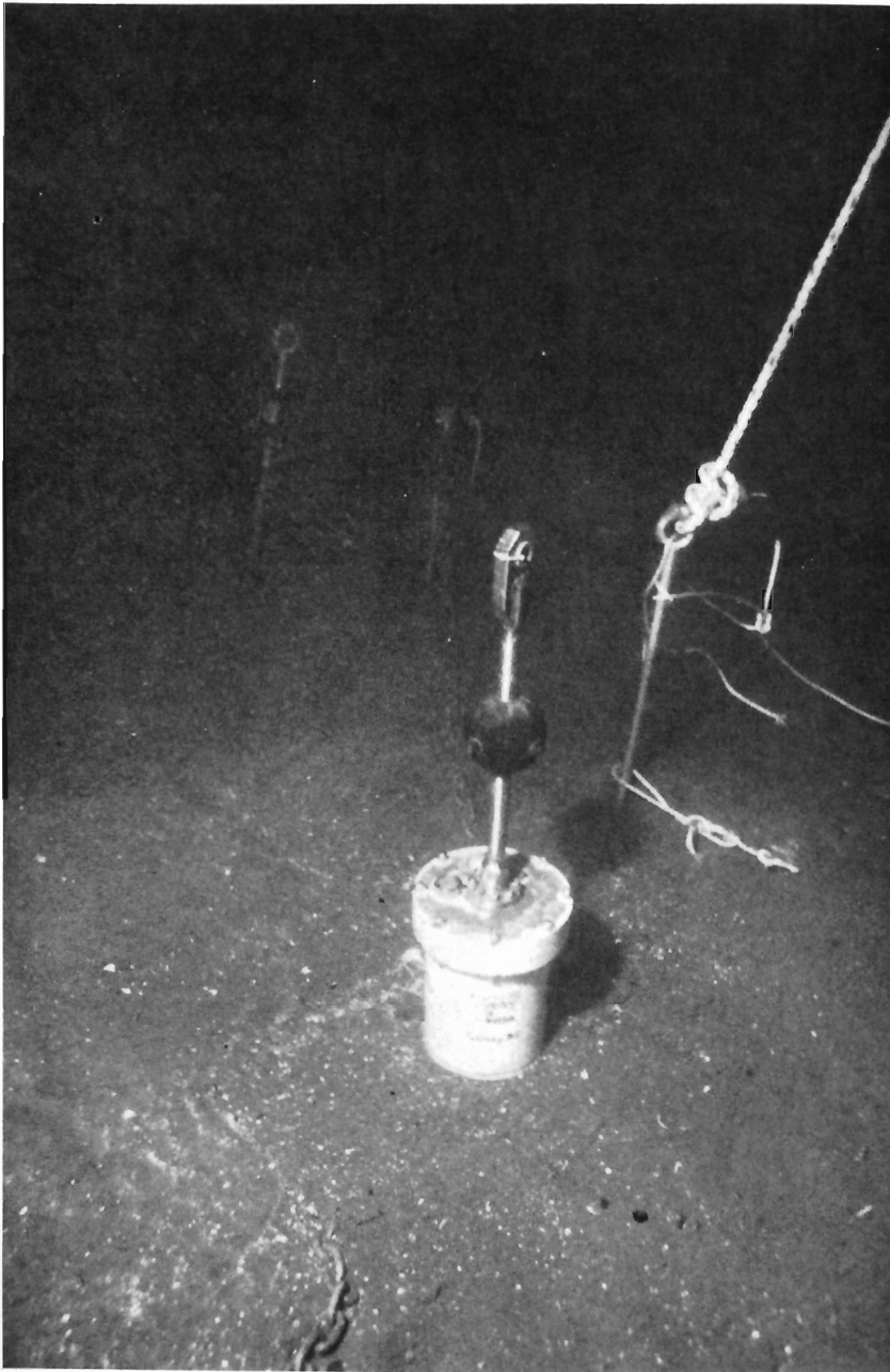
Figure 4. Underwater photograph of the final installation showing the substrate, current meter sensor, and screw anchors. The screw anchor with line attached was used for locating the meter during installation and was removed immediately after the installation. Sensor is 10.2 cm (4 inches) in diameter.
