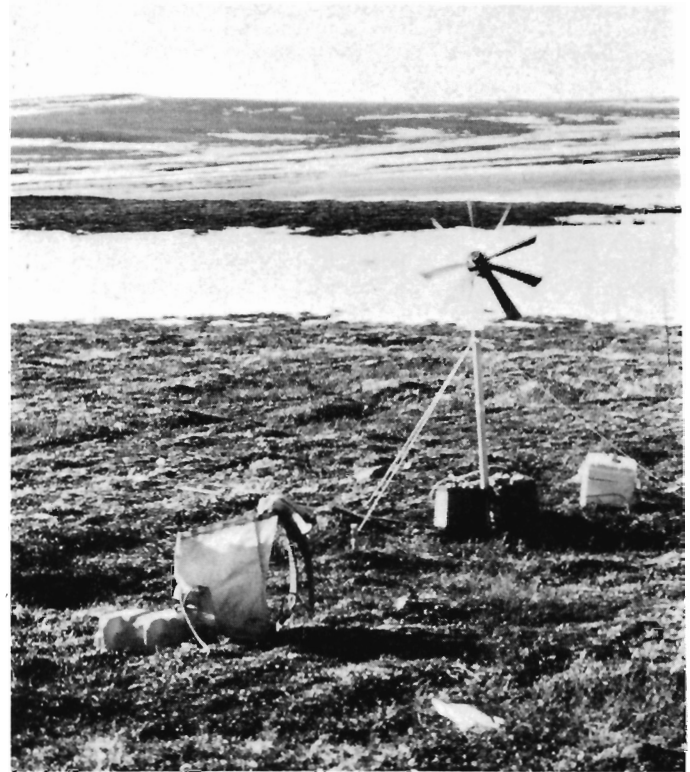
Figure 4. The wind generator in operation, trickle charging uninsulated six volt batteries, North Henik Lake, District of Keewatin.
