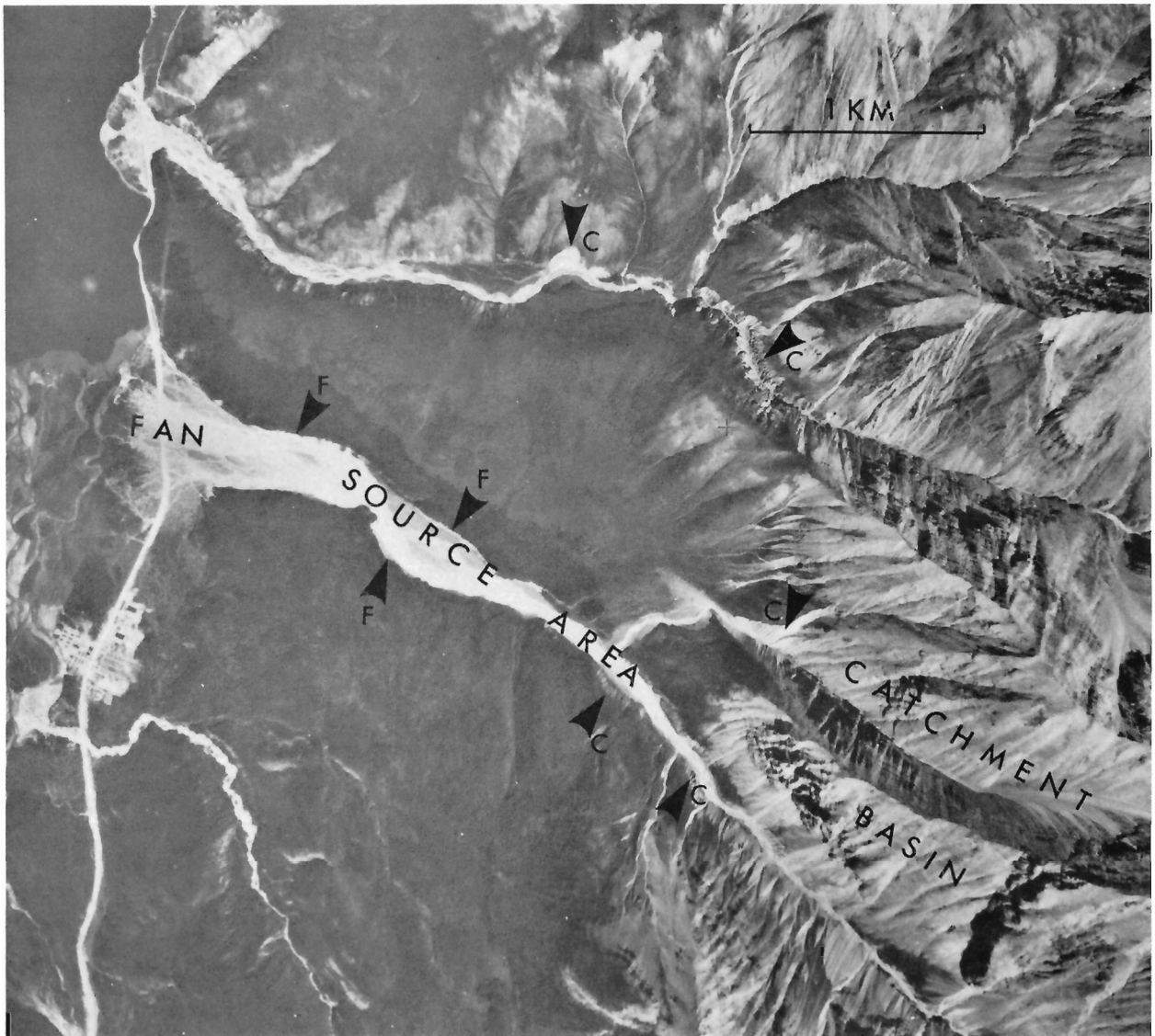
Figure 3.2. Air photo (EMR A 11484/384) of the south end of Muncho Lake, illustrating the complex transition from catchment basin to the debris sources and the depositional fans.
