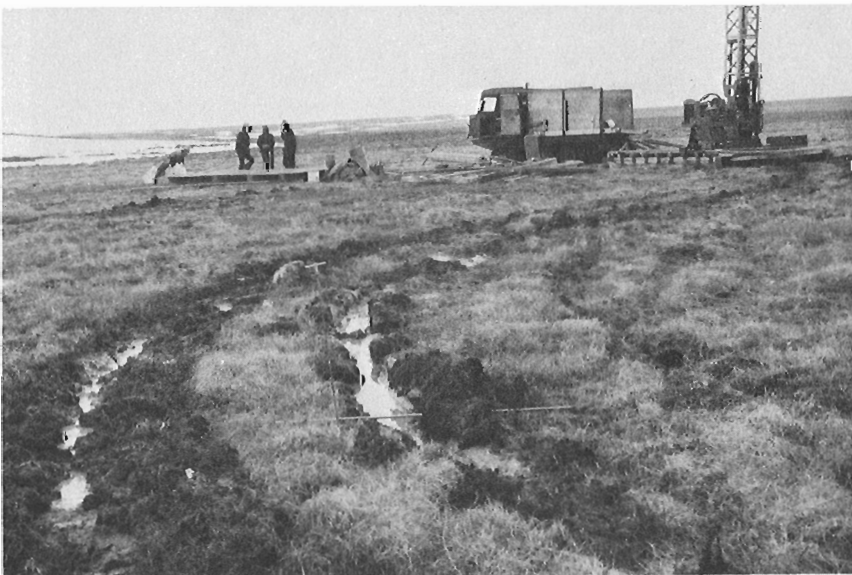
Figure 8.6. An area of rutting associated with sharp turns made by the vehicle moving a drill. The tracks in the foreground were monitored for subsidence by means of bedstead recorder (see text).
