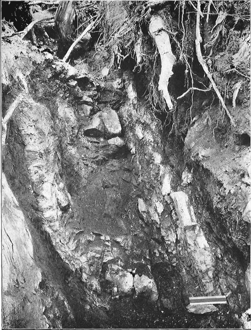
Open-cut at the molybdenite occurrence on Timothy mountain showing two parallel quartz molybdenite veins (white) in quartz diorite. The scale is 6\frac{1}{2} inches long. (Pages 92, 94.)
