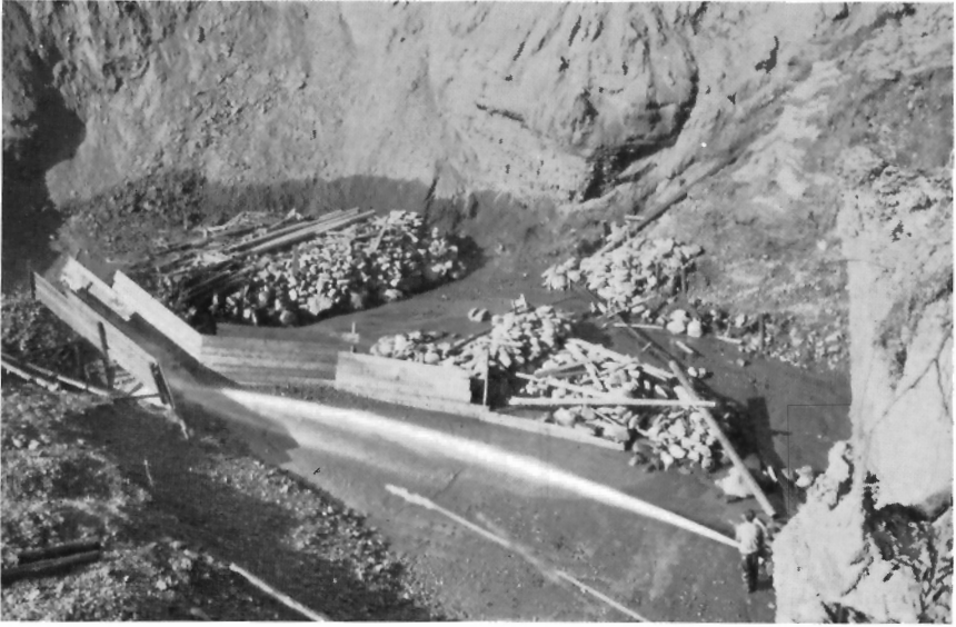
A. Placer workings on Hight Creek. The coarse gravel is swept across the box and the gold and fine material fall through the grating in the bottom of the box into the sluice-boxes.
