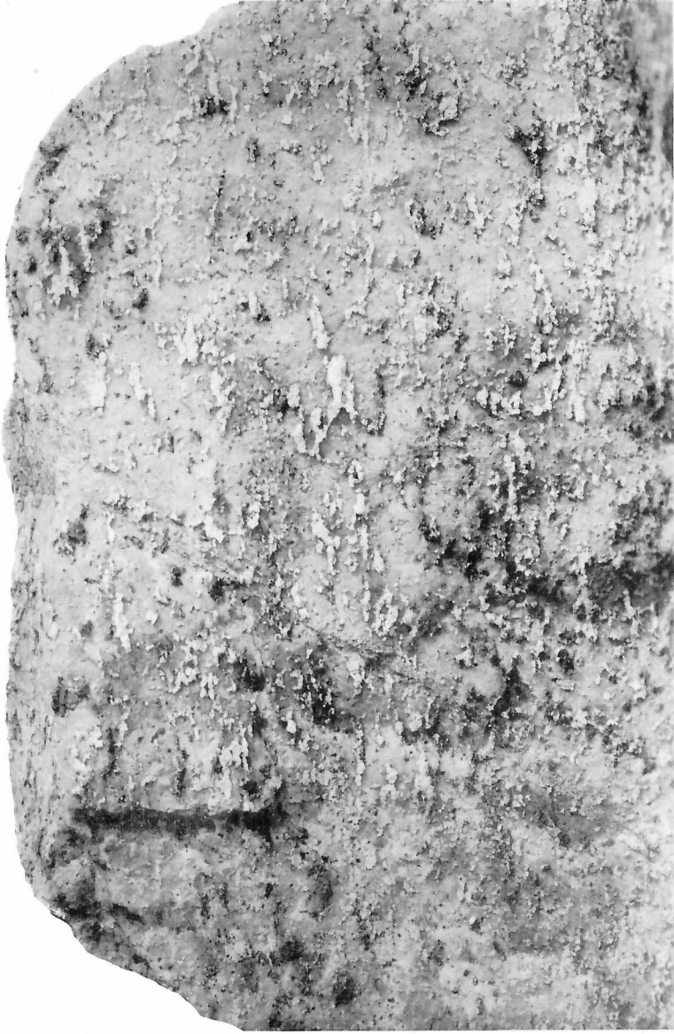
Monmouthite—Township of Monmouth, Lot 11, Concession VIII. Nepheline with subordinate Albite (white) and Hastingsite (black) x \frac{1}{2}
