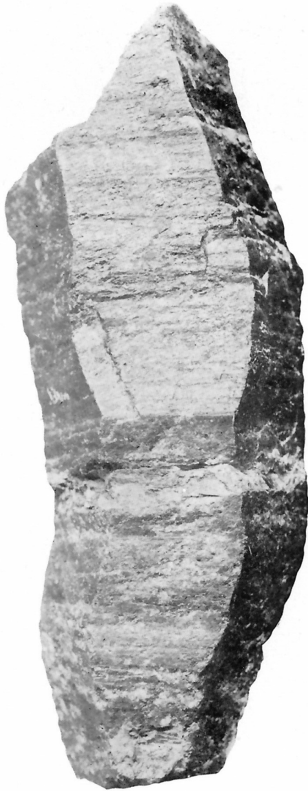
Crystal of Corundum (measures 7 x 2½ inches) showing Muscovite developed along basal parting plane. Craigmont, Raglan township, Ontario.
