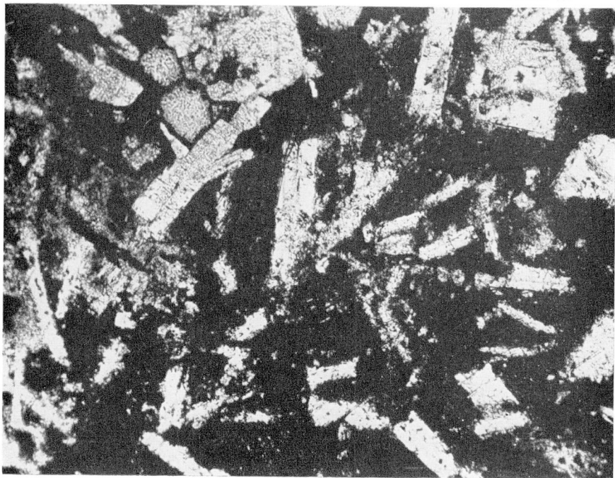
A. Photomicrograph of altered meta-basalt, RA claim group. Black areas consist largely of hematite dust, white rectangular areas are feldspar laths, and light grey areas are aggregates of chlorite and calcite. Plane light.
