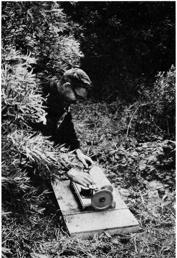
PLATE II Typical observation well with Leupold Stevens type F recorder, placed on a plywood platform.
