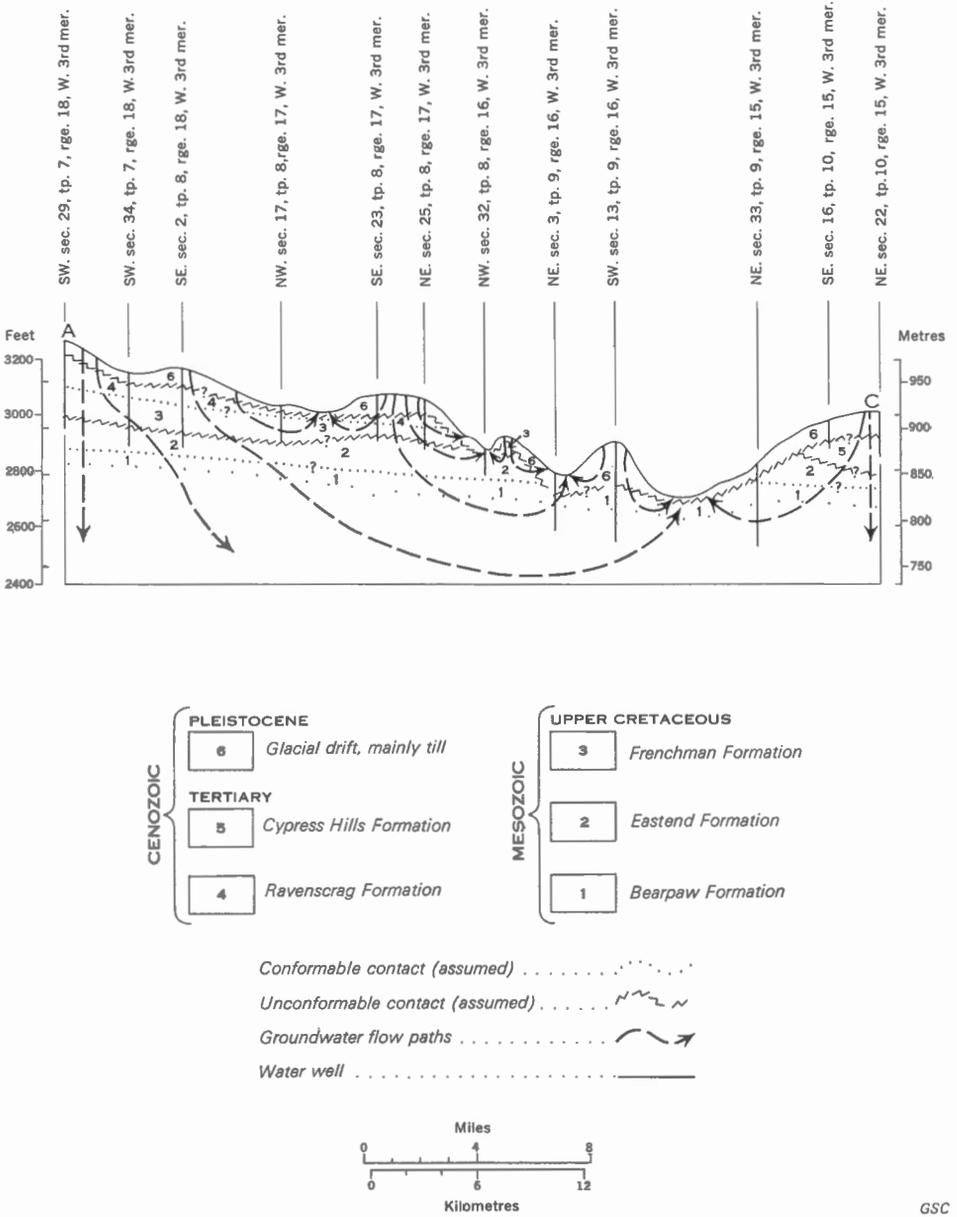
Figure 4. Geological cross-section showing generalized pattern of groundwater flow. For location of section see Figure 2.
