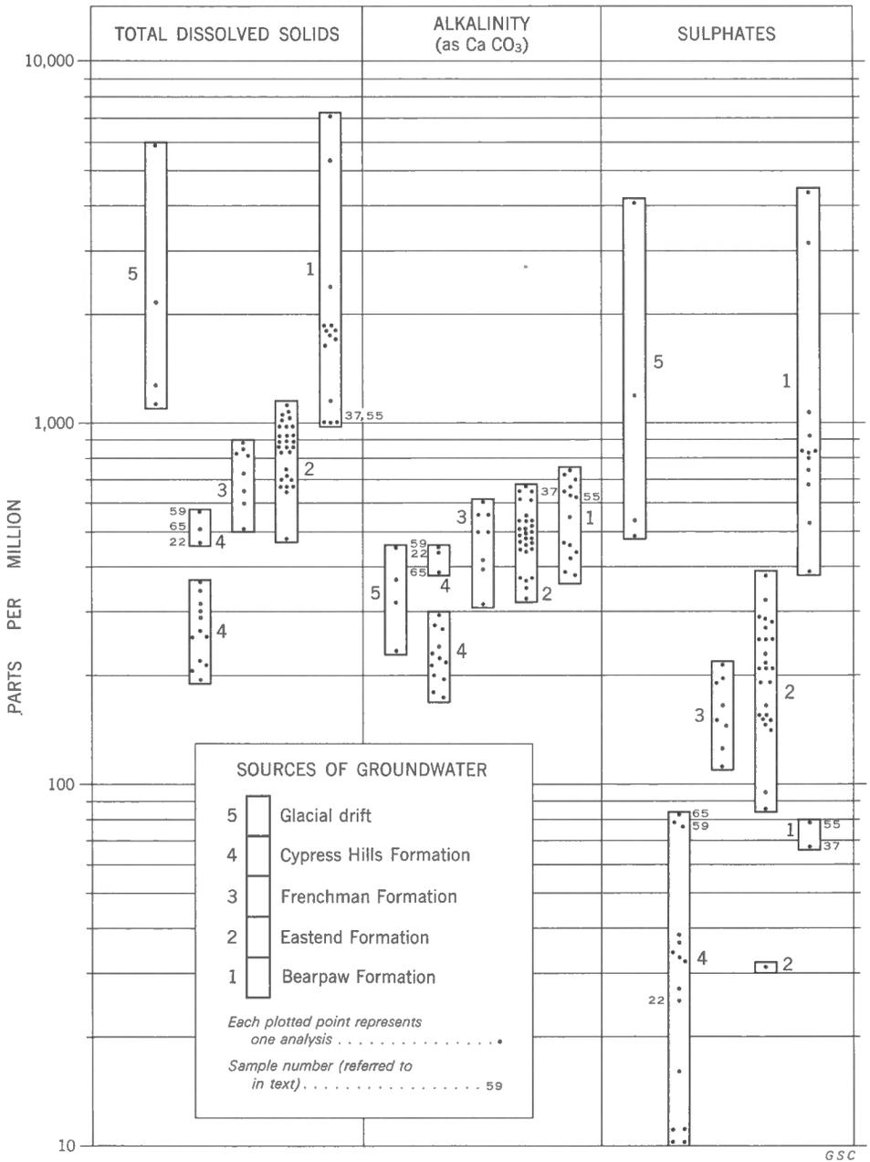
Figure 7. Bar graph comparing total dissolved solids, alkalinity and sulphates of groundwaters of the upper Notukeu Creek basin, southwestern Saskatchewan.
